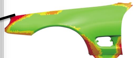
Figure 8. Process capability Cpk, with respect to defined tolerance limits for acceptable springback
