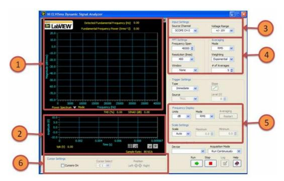
Fig. 9. DSA SFP with important controls labeled
