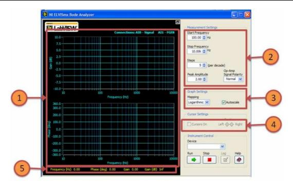
Fig. 8. Bode SFP with important controls labeled
