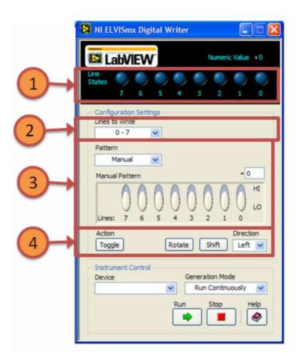
Fig. 12. Digout SFP with important controls labeled
