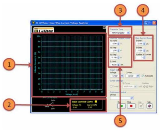
Fig. 15. 3-Wire SFP with important controls labeled
