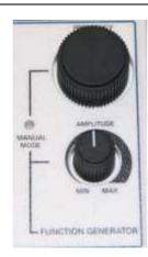
These knobs allow the user to manually adjust the frequency and amplitude for a function generator output waveform. The Manual Mode LED lights up when the function generator is in manual mode.
