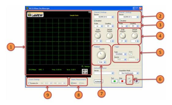
Fig. 5. SCOPE SFP with important controls labeled
