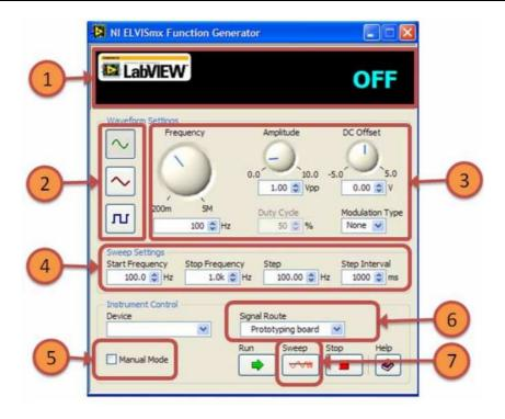
Fig. 6. FGEN SFP with important controls labeled
