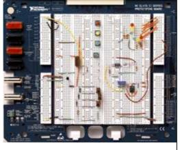
Provides an area for building circuitry and has necessary connections to access signals for common applications
