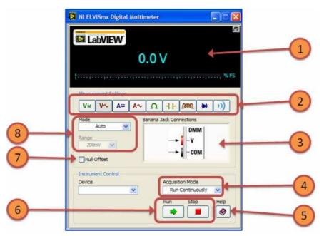
Fig. 4. DMM SFP with important controls labeled
