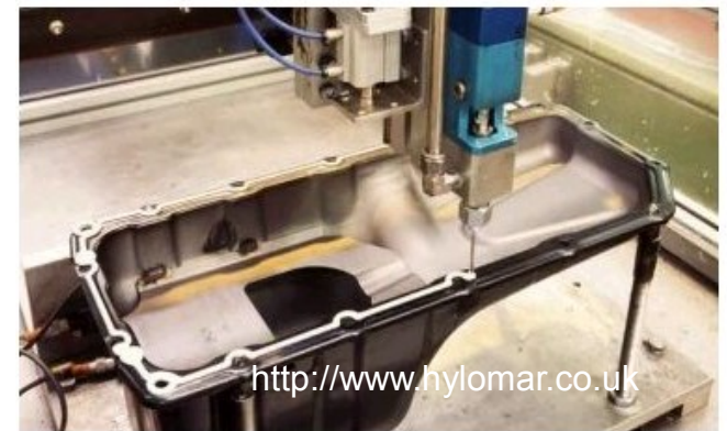
Motor engine sealed with a silicone adhesive
