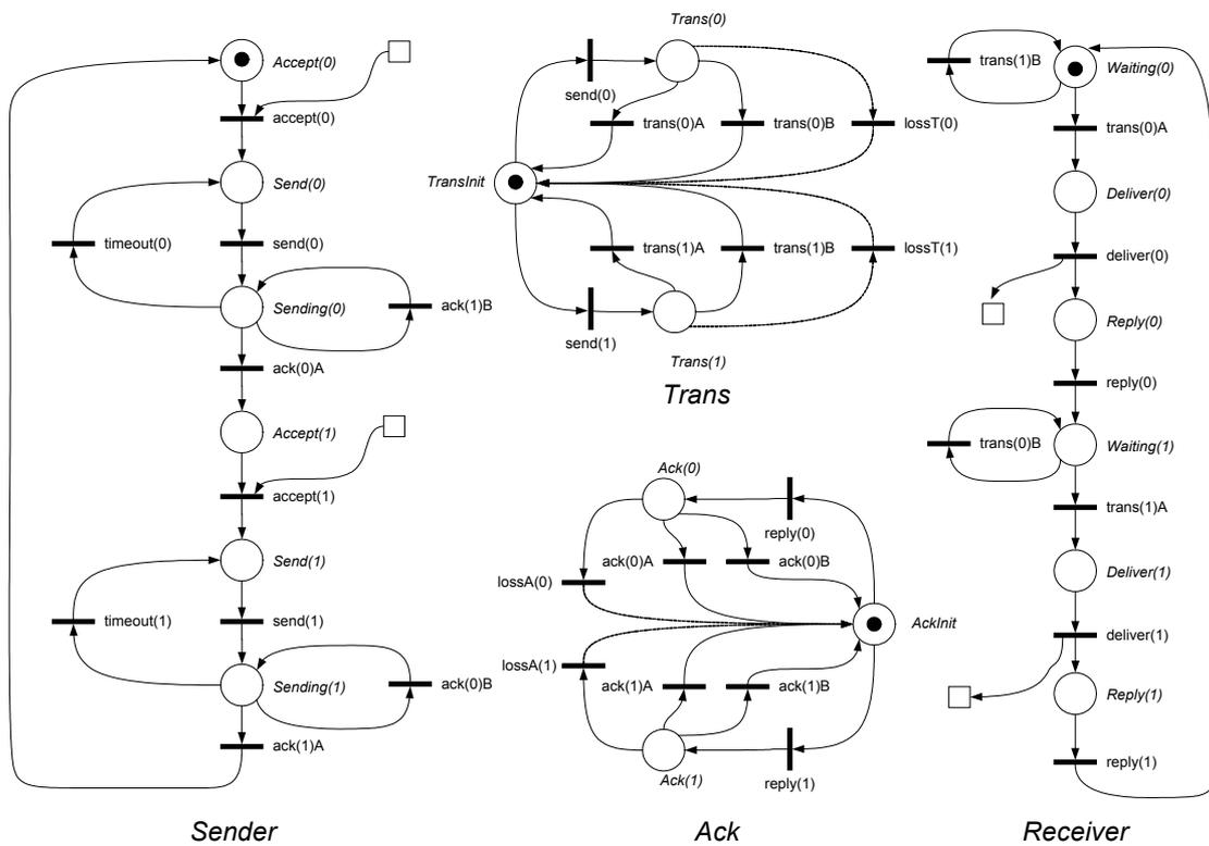
Fig. 4 Verified Petri net modeling alternating bit protocol
