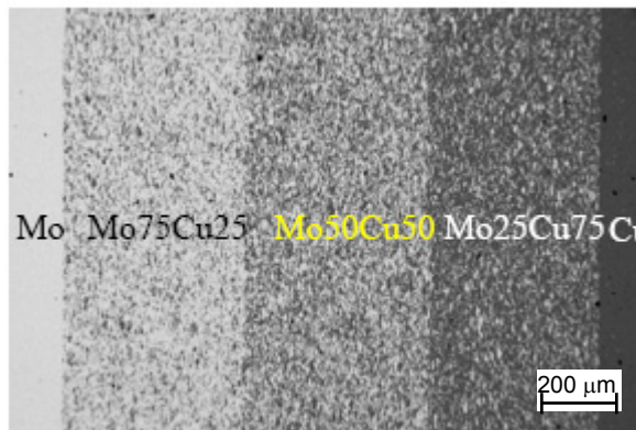
Fig. 21. SEM micrograph of well-sintered Mo/Cu FGM (Ref. [45]).
