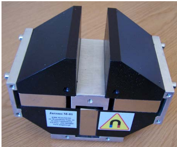
Figure 10. View of the constant magnet used in experiments. The operating space is 0.10×0.05×0.04 m (courtesy of FRI)
