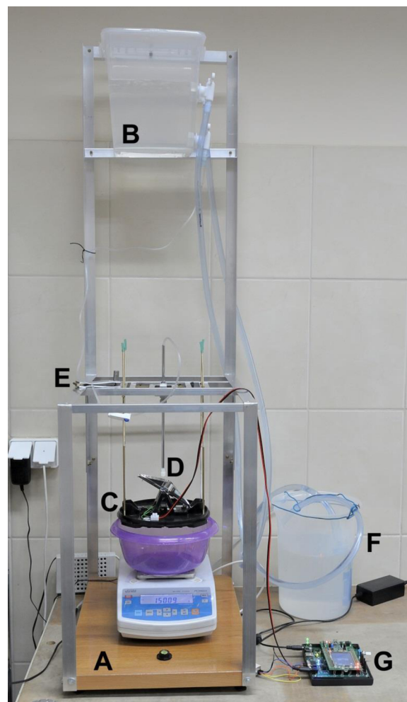
Fig. 1. The laboratory stand used in the calibration process. Flow rate was regulated by a precision clamping screw. The constant difference between the water head in the main container and the dispensing needle ensured a steady flow rate. Every tipped volume of water was measured by a precision laboratory balance. A data logger recorded both the interval between tips and the tipped water weight (volume). A – level platform with precision laboratory balance; B – main water container with constant head of water; C – tipping bucket mechanism; D – dispensing-needle to supply water; E – precision clamping screw to regulate flow rate; F – auxiliary water canister with small pump; G – data logger.
