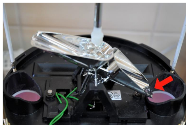
Fig. 8. A large drop formed at the edge of a seesaw-like container as a result of incomplete water outpour.
