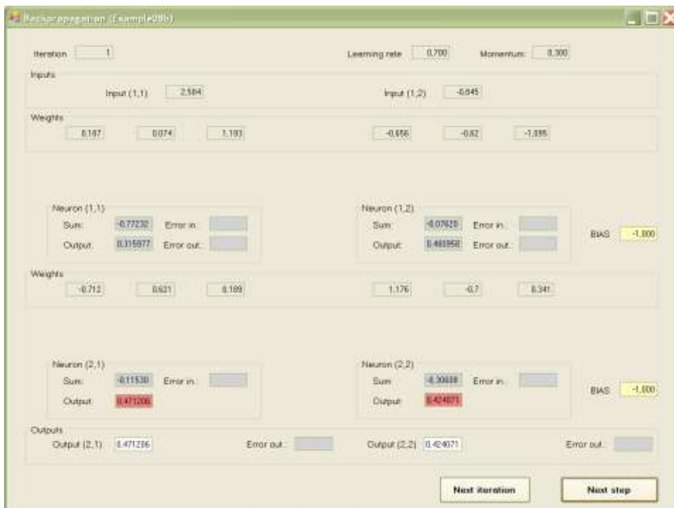
Fig. 7.14. Network after finishing the stage of forward propagation
