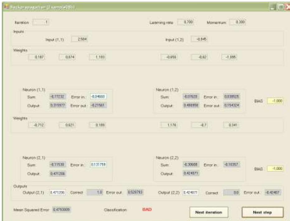
Fig. 7.18. The result of the backpropagation of errors
