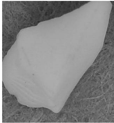
Fig.2. Exterior grit Cubitron (CB) with submicrocrystalline sintered alumina [1]
