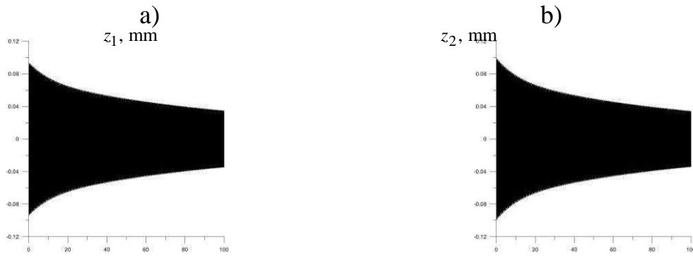
Fig. 9 Displacement of a plate cylinder z_1(t) (a) ) and a blanket cylinder z_2(t) (b) for k_{12}=10 \cdot 10^6 \text{ Nm}^{-1} , \Omega_1=233,468 \text{ s}^{-1} , \Omega_2=388,932 \text{ s}^{-1} , n=5 , \omega=(2 \times 388,932/5) \text{ s}^{-1}=86,4923 \text{ s}^{-1}
