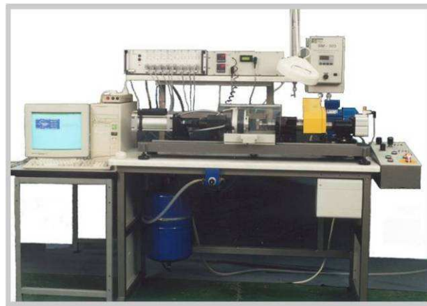
Fig. 1. The testing device for mechanical seals – SUM-1.
