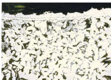
Fig. 3. Microstructure of the superficial layer on steel 3. Mode CTT: 570°; 10 hours, x 200
