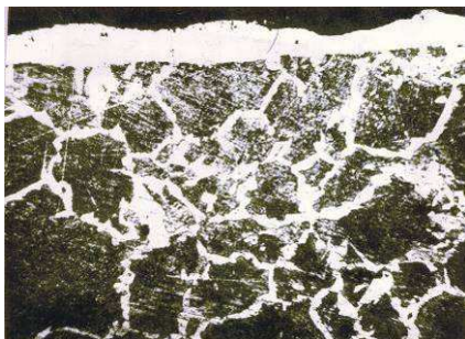
Fig. 1. Microstructure of the superficial layer on steel 20, x 200
