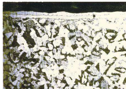
Fig. 2. Microstructure of the superficial layer on steel 3. Mode CTT: 580 °; 3 hours, x 200
