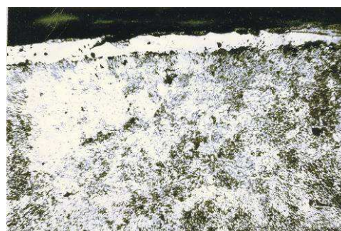
Fig. 4. Microstructure of the superficial layer on steel 40X, x 200
