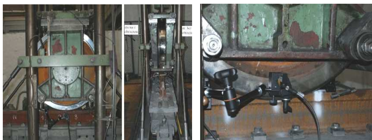
Fig. 2. Laser measurement of wheel plate and wheel/rail contact stiffness.
