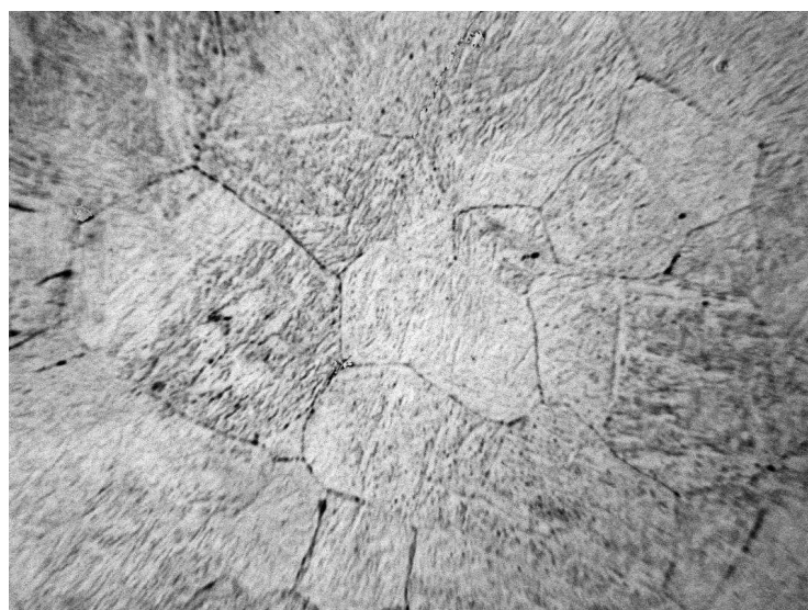
Fig. 4 The microstructure after quenching of X12Cr13 steel (500x)
