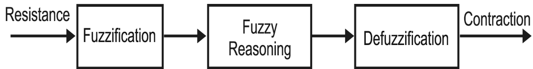
Fig. 2. Block schema of an idea of fuzzy model
