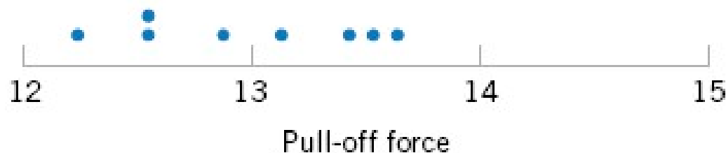
Figure 1-2 Dot diagram of the pull-off force data when wall thickness is 3/32 inch.
