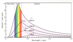
The **total energy density** (the energy density integrated over all frequencies) for the blackbody radiation is a function of the temperature alone:
