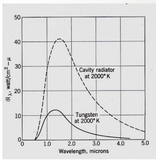
The spectral radiancy of tungsten (ribbon and cavity radiator) at 2000 K.
