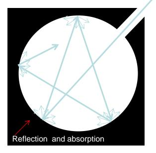
A small hole cut into a cavity is the most popular and realistic example of the blackbody.
