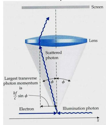
Suppose an electron moves from the left to the right with the well-defined initial momentum  $p_x$ . The electron's position is to be observed by shining light on it.
