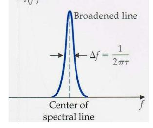
Broadening of spectral lines is a quantum mechanical phenomenon
