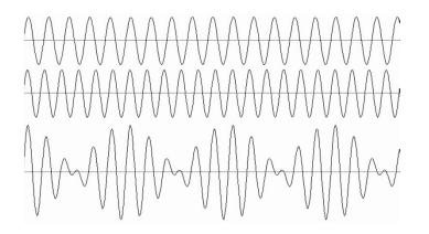
If several waves of different wavelengths (frequencies) and phases are superposed together, one would get a localized wave packet
