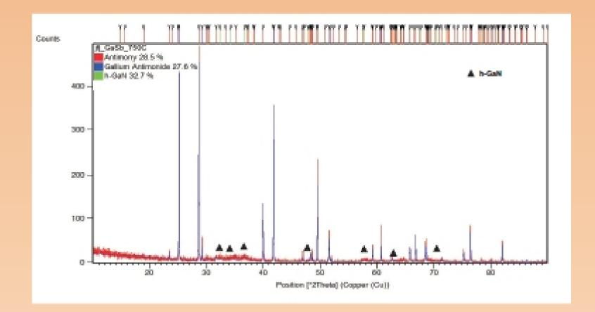
The product powder from the lowest temperature of 750 °C and short reaction timeof 6 h (Sample 1, XRD pattern above) contains some GaN but, also, a proportion of unreacted gallium antimonide GaSb and elemental antimony Sb, a transient by-product. The proportion of nanocrystalline h-GaN in this powder was estimated at *ca.* 33 %.
