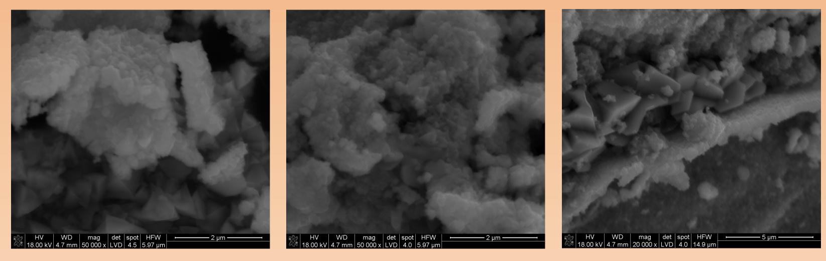
The fully reacted powders (Samples 2-5) were represented by two dominant morphologies. The pyramidal blocky nanocrystallites were observed in Sample 3 containing exclusively the h-GaN polytype. For Samples 2, 4, and 5 consisting of both polytypes, the pyramids were accompanied by particles with an ill-defined morphology.
