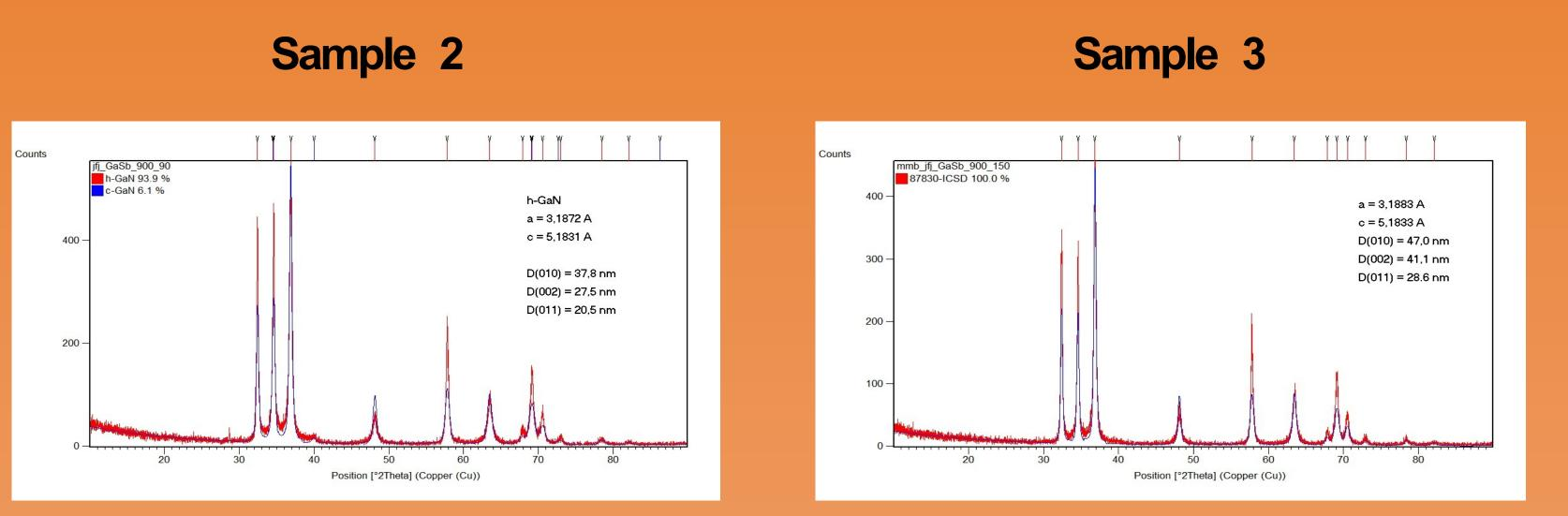
and, following a purge of the system with nitrogen, high purity ammonia was introduced at 1 cm<sup>3</sup>/s. After reaching a selected furnance temperature (range 750-1000 °C) the GaSb powders were nitridated for 6 to 150 hours. The fine yellow product powders were analyzed using the powder XRD and SEM/EDX examination.
