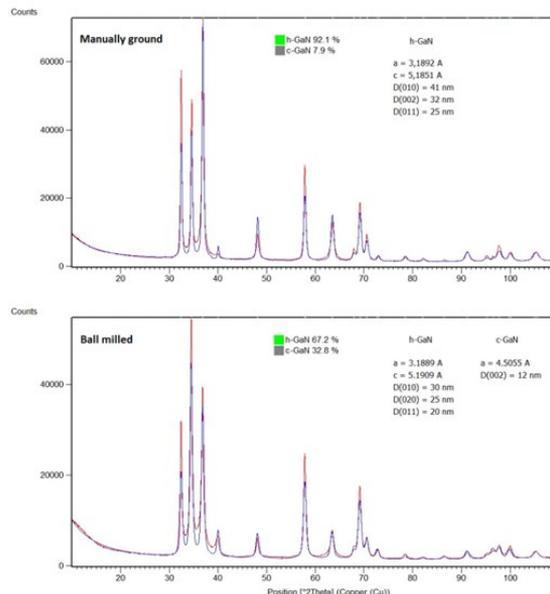
Fig. 2. XRD diffraction patterns for the products from nitridation with  $\text{NH}_3$  at **900 °C, 170 h**, of powdered GaSb; *top* – manually ground, *bottom* – ball milled
