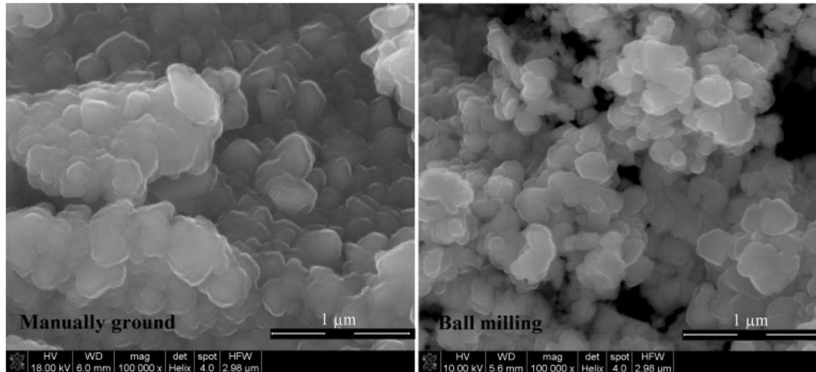
Fig. 9. SEM images of GaN powders prepared at **900 °C, 170 h** from: *left* – manually ground precursor, *right* – ball milled precursor. Note the identical scale bars in both images.
