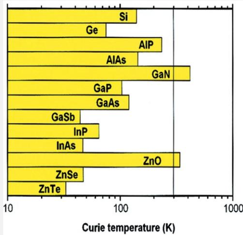
Computed values of the Curie temperature  $T_C$  for various p-type semiconductors containing 5 % of Mn and  $3.5 \times 10^{20}$  holes per  $\text{cm}^3$ .
