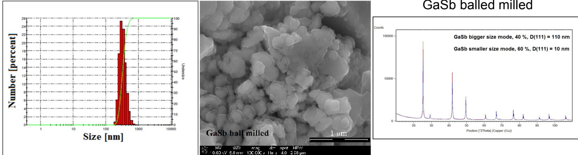
Fig. 6. Ball milled GaSb: *left* – particle size distribution by number, *middle* – SEM image, *right* – XRD spectrum
