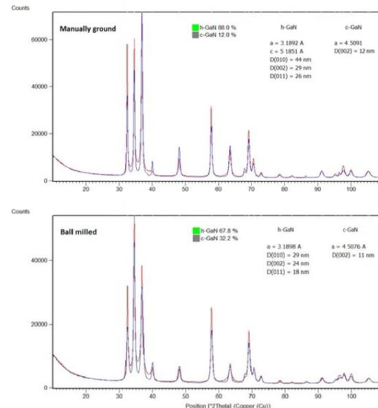
Fig. 3. XRD diffraction patterns for the products from nitridation with  $\text{NH}_3$  at **1000 °C, 36 h**, of powdered GaSb; *top* – manually ground, *bottom* – ball milled
