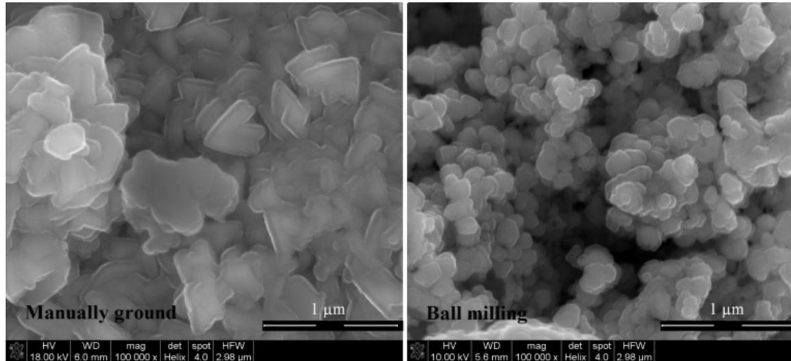
Fig. 10. SEM images of GaN powders prepared at **1000 °C, 36 h** from: *left* – manually ground precursor, *right* – ball milled precursor. *Note the identical scale bars in both images.*
