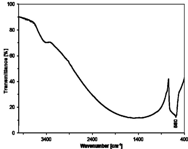
Fig. 5. FT-IR spectrum of the product from nitridation with  $\text{NH}_3$  at **1000 °C, 36 h**, of balled milled GaSb
