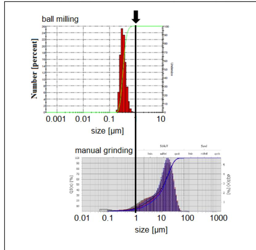
Manual grinding results, relatively, in much wider particle size distribution and significantly bigger particles, on average, some 30 times bigger.
