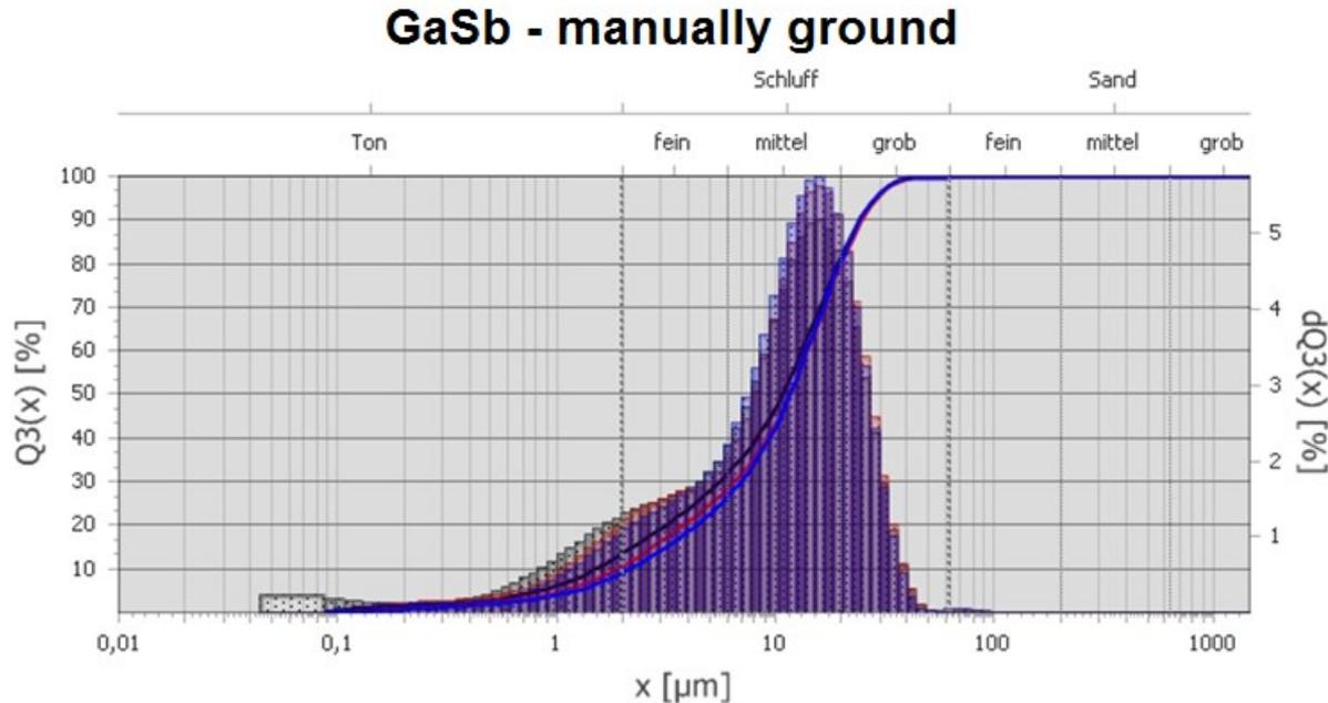
Fig. 7. Particle size distribution by number for manually ground GaSb
