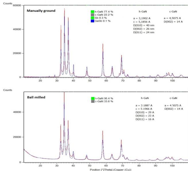
Fig. 1. XRD diffraction patterns for the products from nitridation with  $\text{NH}_3$  at **900 °C, 90 h**, of powdered GaSb; *top* – manually ground, *bottom* – ball milled
