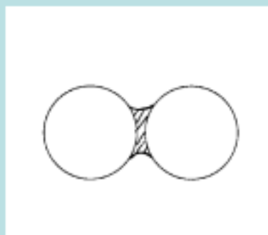
Bridging between two spheres due to capillary condensation
