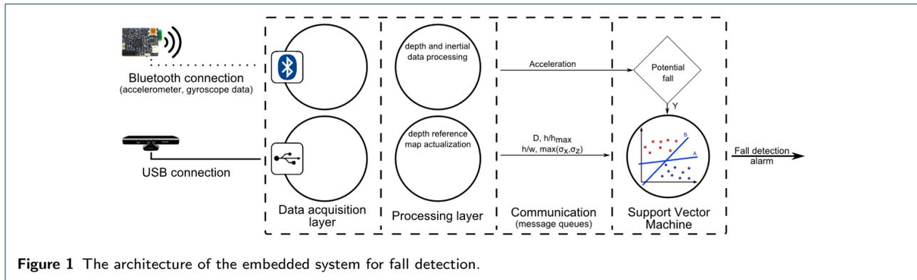
**Figure 1** The architecture of the embedded system for fall detection.
