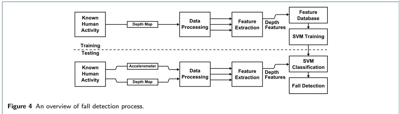
Figure 4 An overview of fall detection process.
