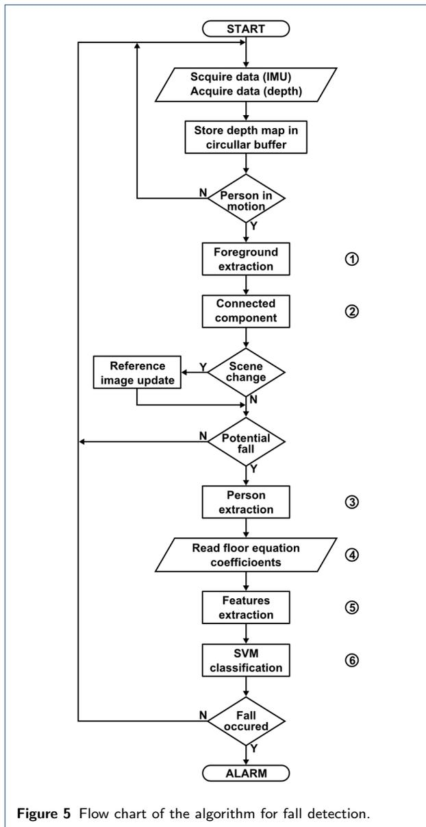
Figure 5 Flow chart of the algorithm for fall detection.
