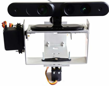
Fig. 3. Depth sensor (Asus Xtion PRO) and our pan-tilt unit.
