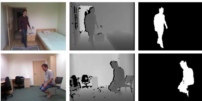
Figure 7: Delineation of person using depth reference image. RGB images (left), depth (middle) and binary images depicting the delineated person (right).
