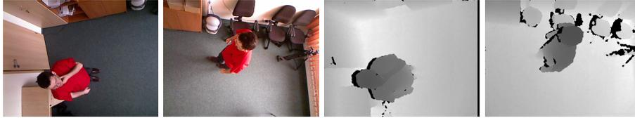
**Fig. 2.** Example top-view images captured by Kinect mounted on pan-tilt head, RGB images (top row), depth images (bottom row).
