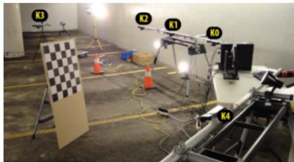
Fig. 2.8: Calibration of multiple Kinect sensors (source: [164]).
