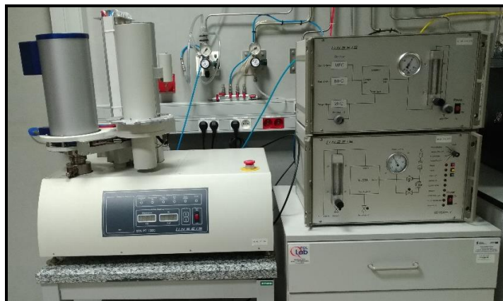
Thermobalance Q5000IR TA Instruments with quadrupole mass spectrometer Pfeiffer Vacuum ThermoStar
