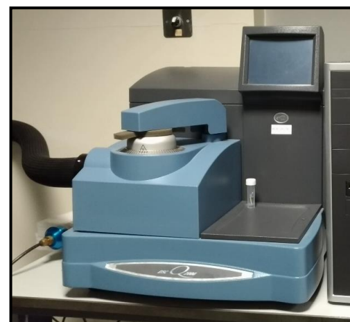
Differential Scanning Calorimeter TA Q2000 allowing measurements 80 to 600 K
