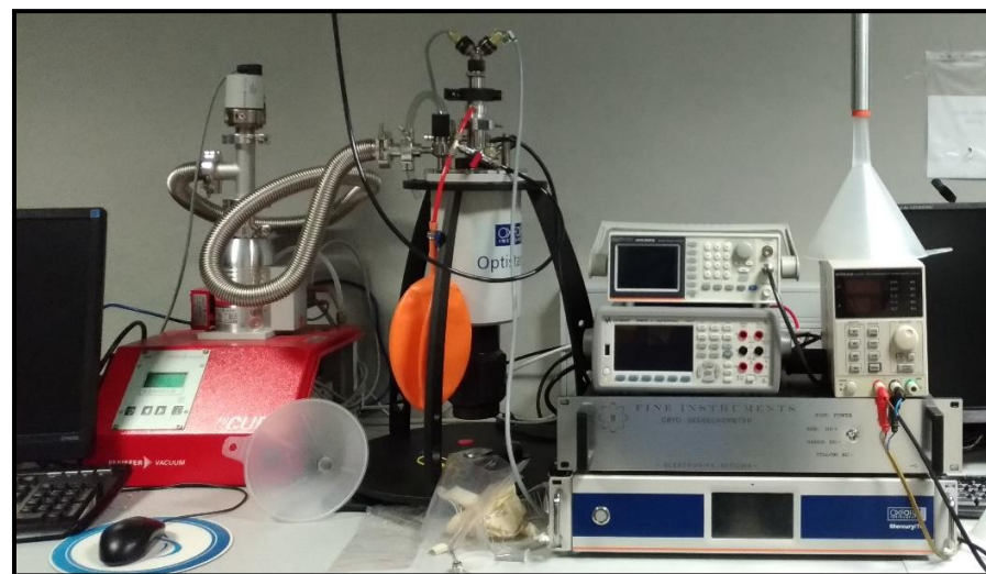
Oxford Cryostat setup, allowing measurements in the range from 20 to 300 K
