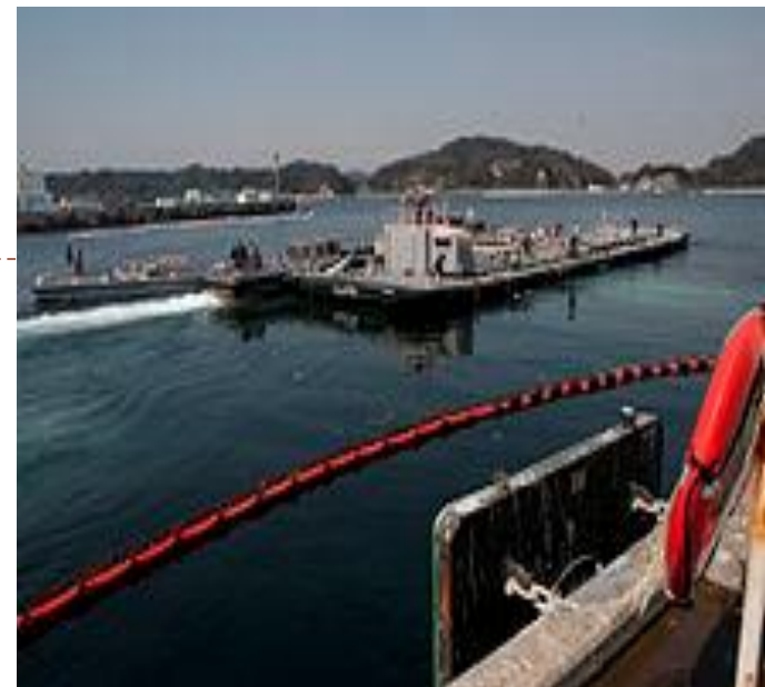
Because of saltwater corrosion problems and pipes clogging by salt, fresh cooling water is transported by barge to Fukushima
