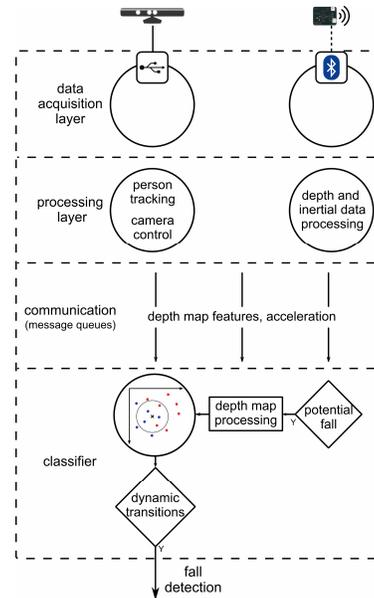
Fig. 5. Data acquisition, processing and communication between the main processes.
