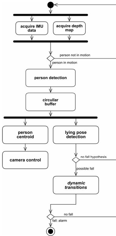
Fig 5. Data processing (UML diagram)
