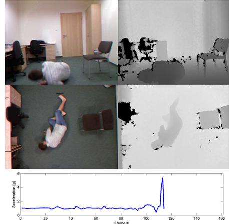
Fig 6. Sample images from the UR Fall Detection dataset with corresponding plot of the acceleration vs. time.
