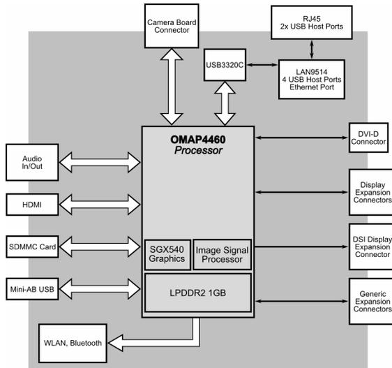
Fig. 4. Block diagram of the PandaBoard ES.
