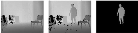
Fig. 1. Person extraction in frontal depth maps. Depth reference image (left), current image (middle), image with the extracted person (right).
