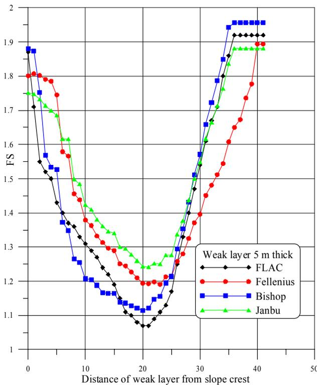
Figure 5. FS values for a 5.0 m thick weak layer.
