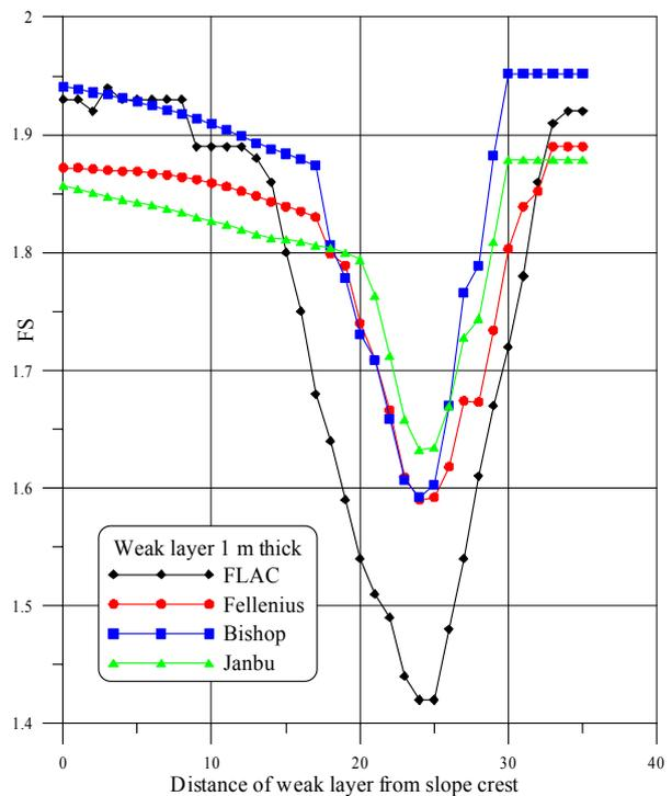
Figure 4. FS values for a 1.0 m thick weak layer.
