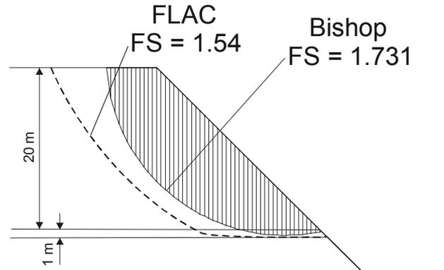
Figure 6. Critical slip surfaces identified by SSR and LEM.
