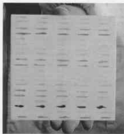
Figure 1 A precursor library including 100 samples on a palm-sized alumina plate.
