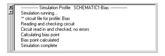
Figure 2-6 PSpice simulation output window.
