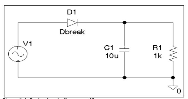
Figure 4-4 Design for a half-wave rectifier.
