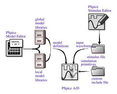
Figure 1-1 User-configurable data files that PSpice A/D reads.
