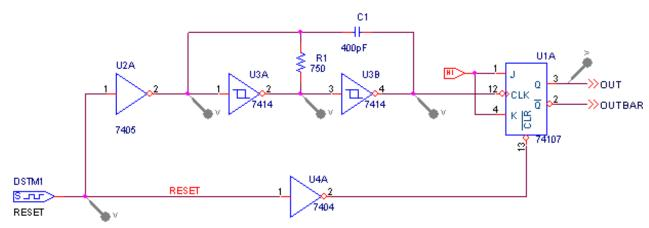
Figure 17-8 Mixed analog/digital oscillator
