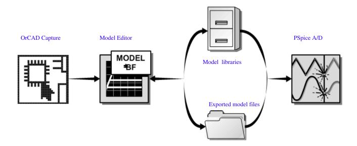
Figure 4-1 Relationship of the Model Editor to design entry tool and PSpice.
