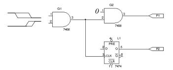
Figure 14-3 Circuit with a timing ambiguity
