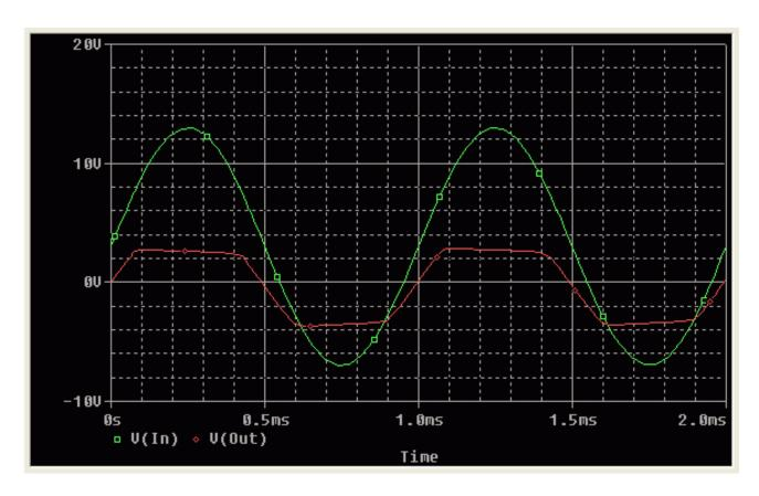
Figure 2-19 Sinusoidal input and clipped output waveforms.
