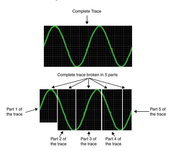
Figure 17-3 Displaying partial traces
