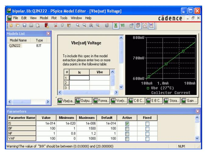
All the PSpice Model Editor needs is information about the device found in standard data sheets. As you enter the data sheet information, the Model Editor displays device characteristic curves so you can verify the model-based behavior of the device. When you are finished, the PSpice Model Editor automatically creates a part for the model so you can use the modeled part in your design immediately.
