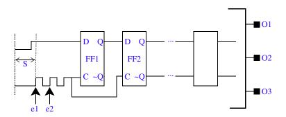
Figure 14-2 Circuit with a timing error.
