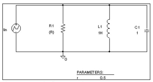
Figure 11-1 Passive filter schematic.
