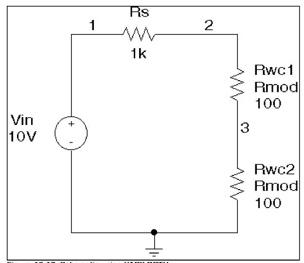
Figure 13-17 Schematic using VARY BOTH.
