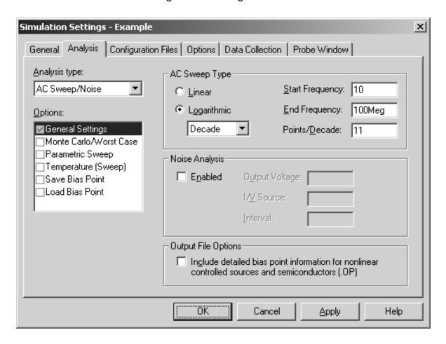
Figure 2-22 AC sweep and noise analysis simulation settings.
