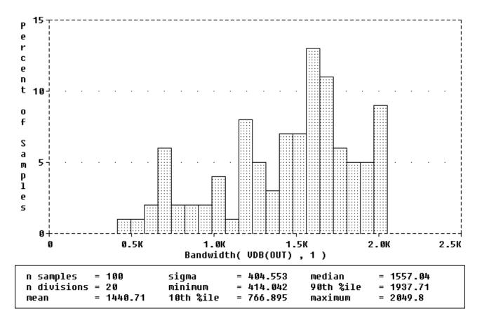
Figure 13-9 1 dB bandwidth histogram.
