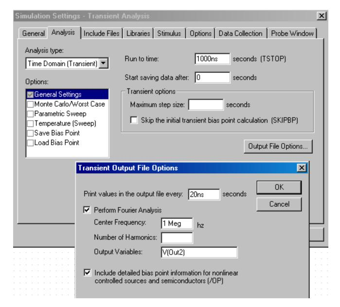
Figure 12-1 Transient analysis setup for EXAMPLE.OPJ.
