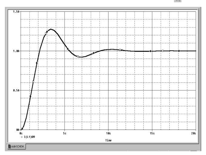
Figure 11-2 Current of L1 when R1 is 1.5 ohms.
