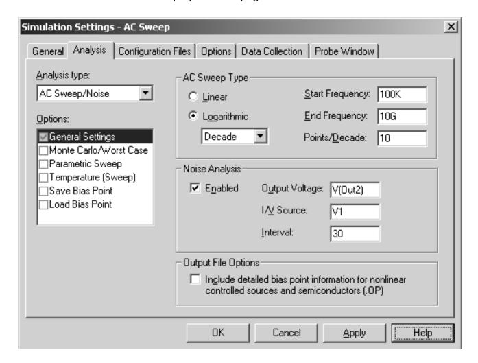
Figure 10-2 AC analysis setup for EXAMPLE.OPJ.
