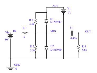
Figure 2-5 Diode clipper design
