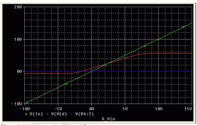
Figure 2-11 Voltage at In, Mid, and Out.
