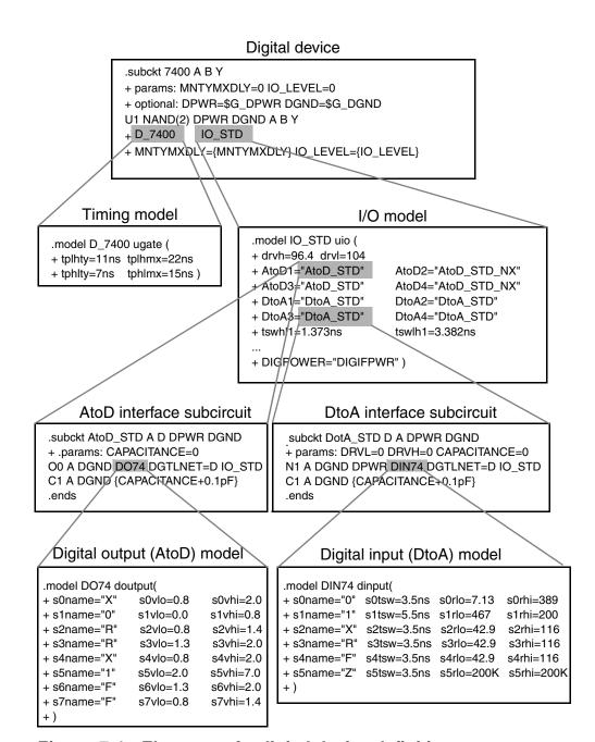
Figure 7-1 Elements of a digital device definition
