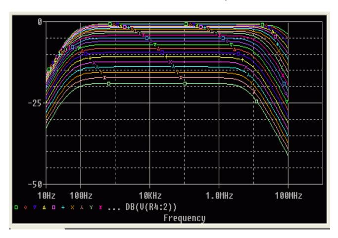
Figure 2-28 Small signal response as R1 is varied from 100 $\Omega$  to 10 k $\Omega$ .
