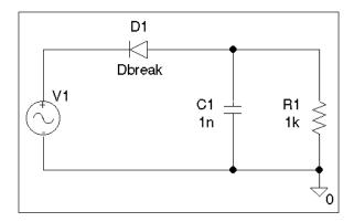
Figure 4-5 Design for a half-wave rectifier.
