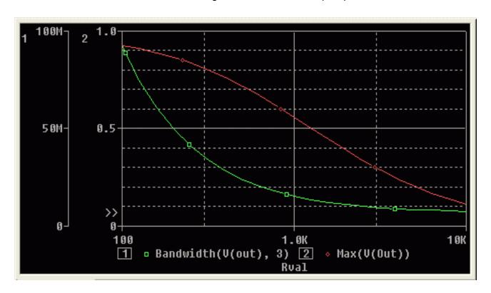
Figure 2-30 Performance analysis plots of bandwidth and gain vs. Rval.
