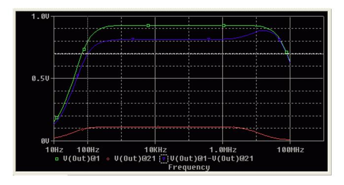
Figure 2-29 Small signal frequency response at 100 and 10  $k\Omega$ input resistance.
