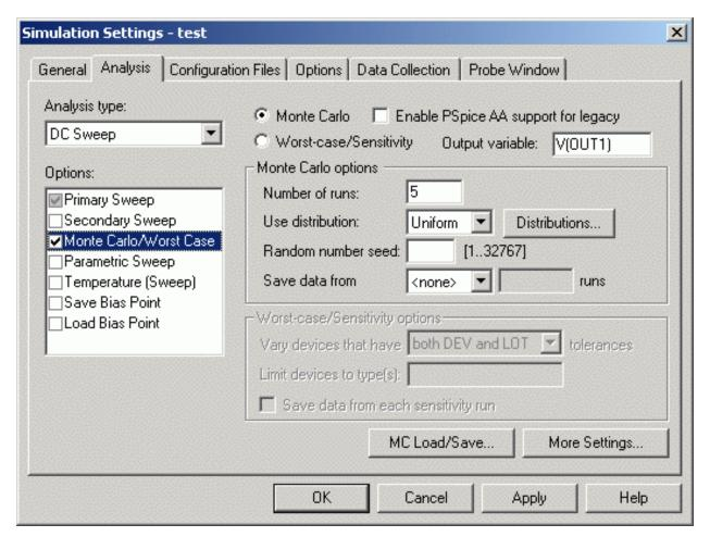
Figure 13-2 Monte Carlo analysis setup for EXAMPLE.OPJ.
