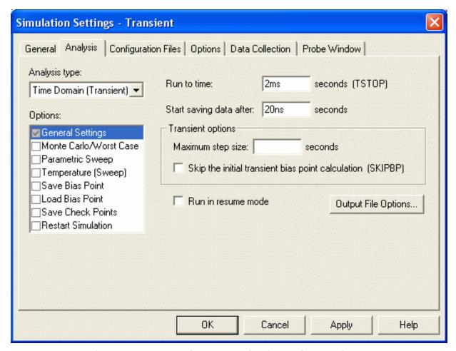
Figure 2-18 Transient analysis simulation settings.
