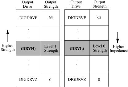
Figure 7-2 Level 1 and 0 strength determination.
