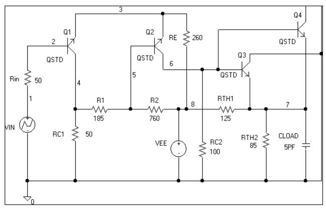
Figure 12-3 ECL-compatible Schmitt trigger.
