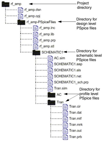
Figure 1-2 Directory structure of RF\_AMP analog project
