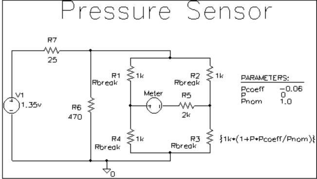
Figure 13-5 Pressure sensor circuit.
