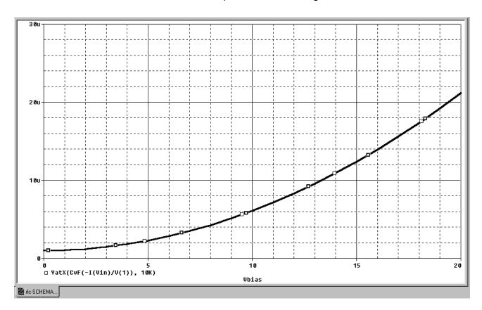
Figure 11-5 Plot of capacitance versus bias voltage.
