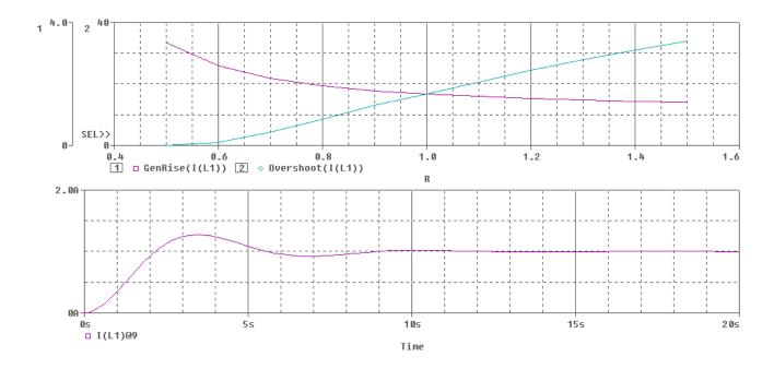
Figure 11-3 Rise time and overshoot vs. damping resistance.
