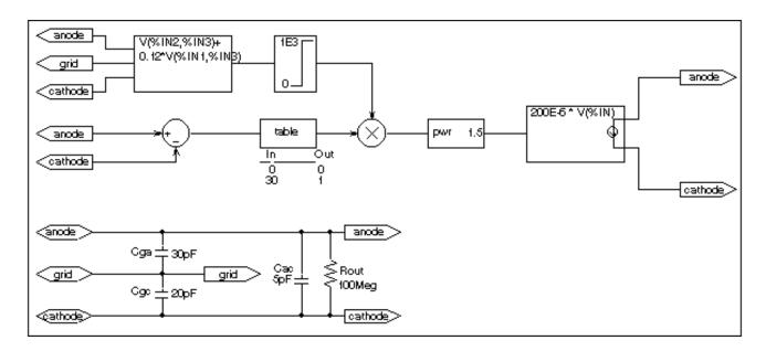
Figure 6-13 Triode circuit.
