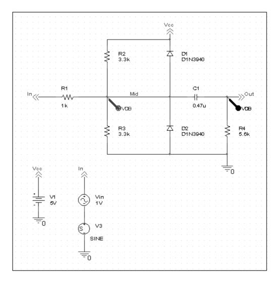
Figure 2-20 Clipper circuit with AC stimulus in capture.
