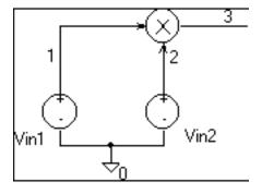
Figure 6-20 Voltage multiplier circuit (mixer).
