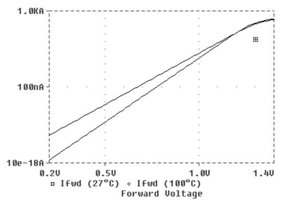
Figure 4-8 Forward Current device curve at two temperatures.
