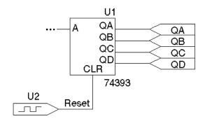
Figure 14-1 FILESTIM1 used on a schematic page.
