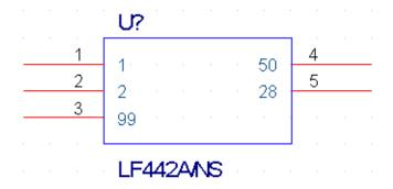
Instead of a regular triangular graphic, a rectangular graphic is generated. The numbers inside the rectangle are the pin names and the numbers outside the rectangle represent pin numbers.
