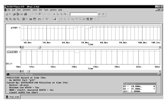
Figure 17-12 Waveform display for a persistent hazard.
