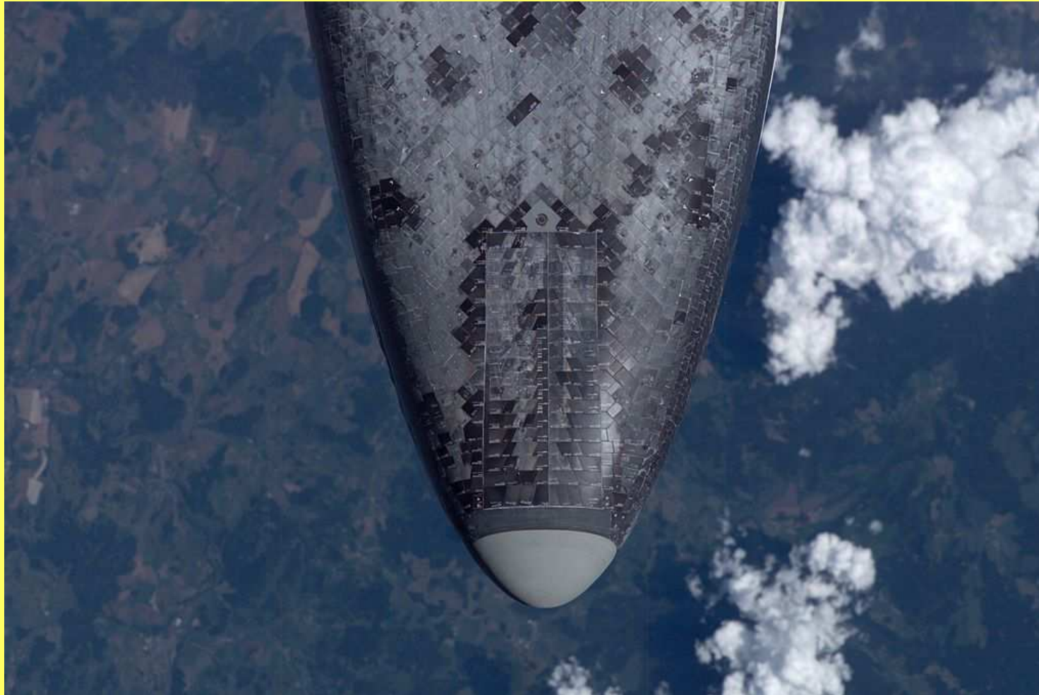
Thermal soak aerodynamic heat shield used on a Space Shuttle
