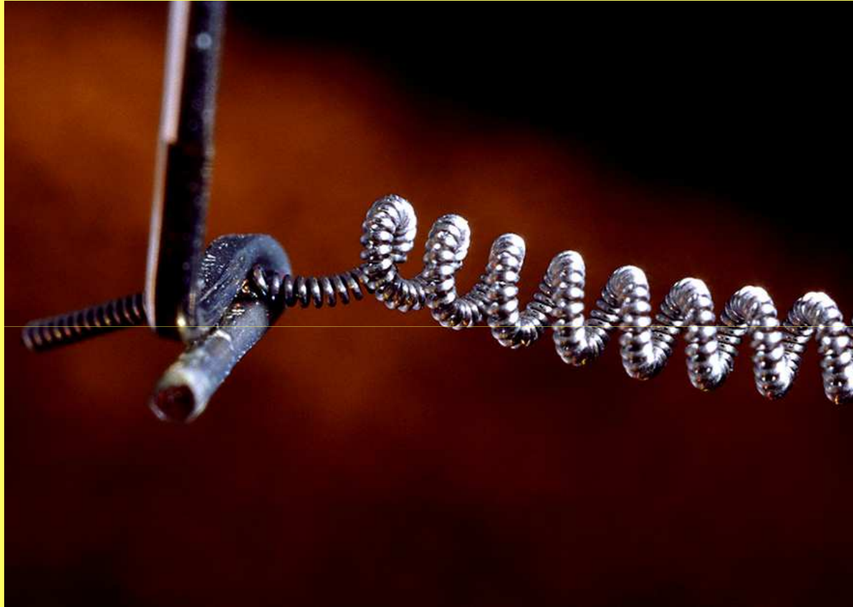
Filament of a 200 Watt incandescent lightbulb
