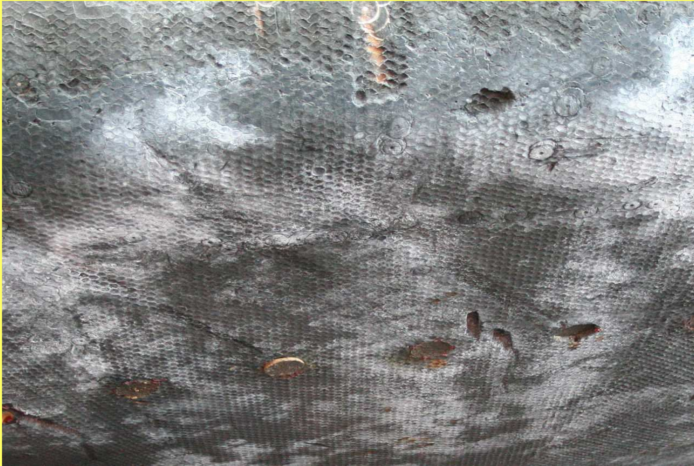
Apollo 12 capsule's ablative heat shield (after use)
