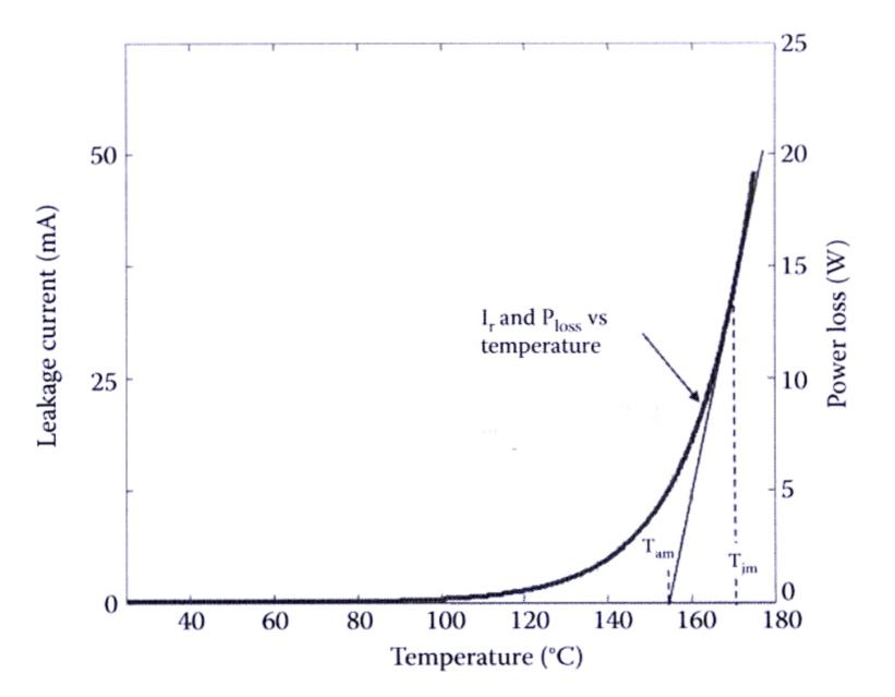
Power loss in *p*-*n* Si diode induced by leakage current.
