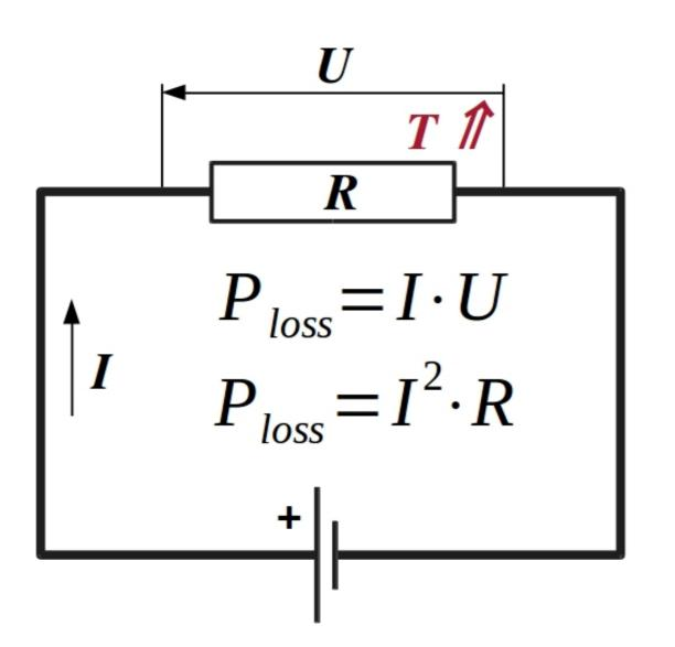
P<sub>loss</sub> – electric power loss in the component
