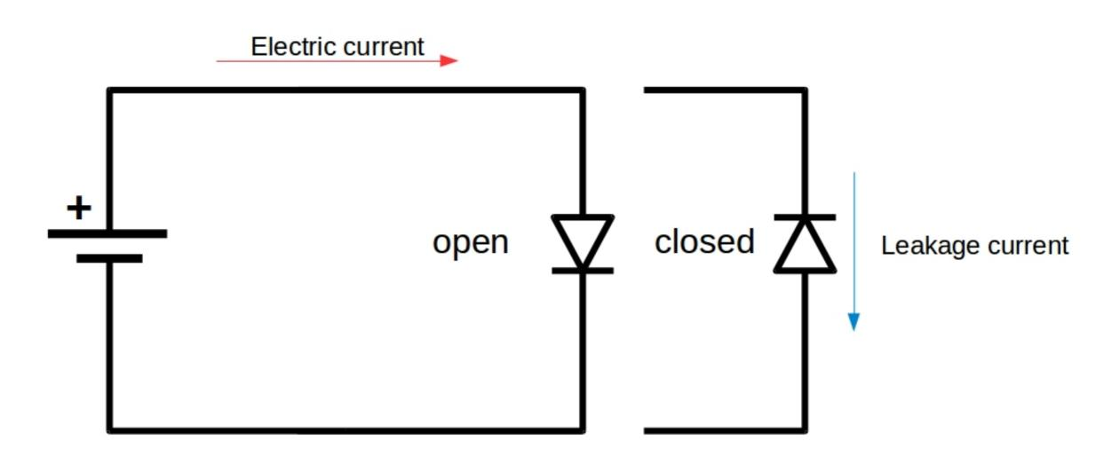
*p-n* junction diode works like electric one-way valve
