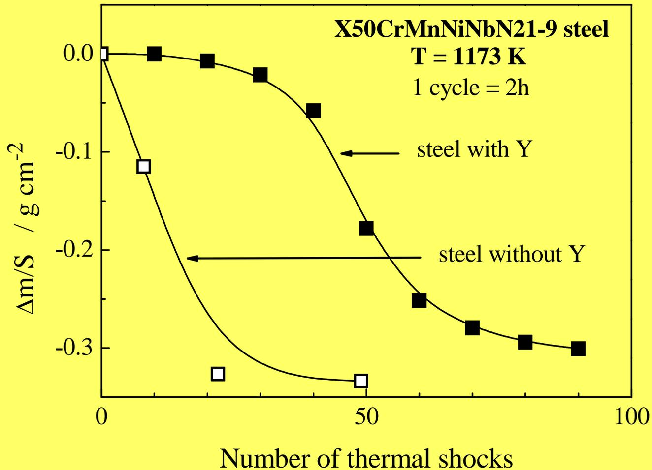
Corrosion behaviour of the X53CrMnNiN20-8 steel uncovered and covered with yttrium under thermal shock conditions
