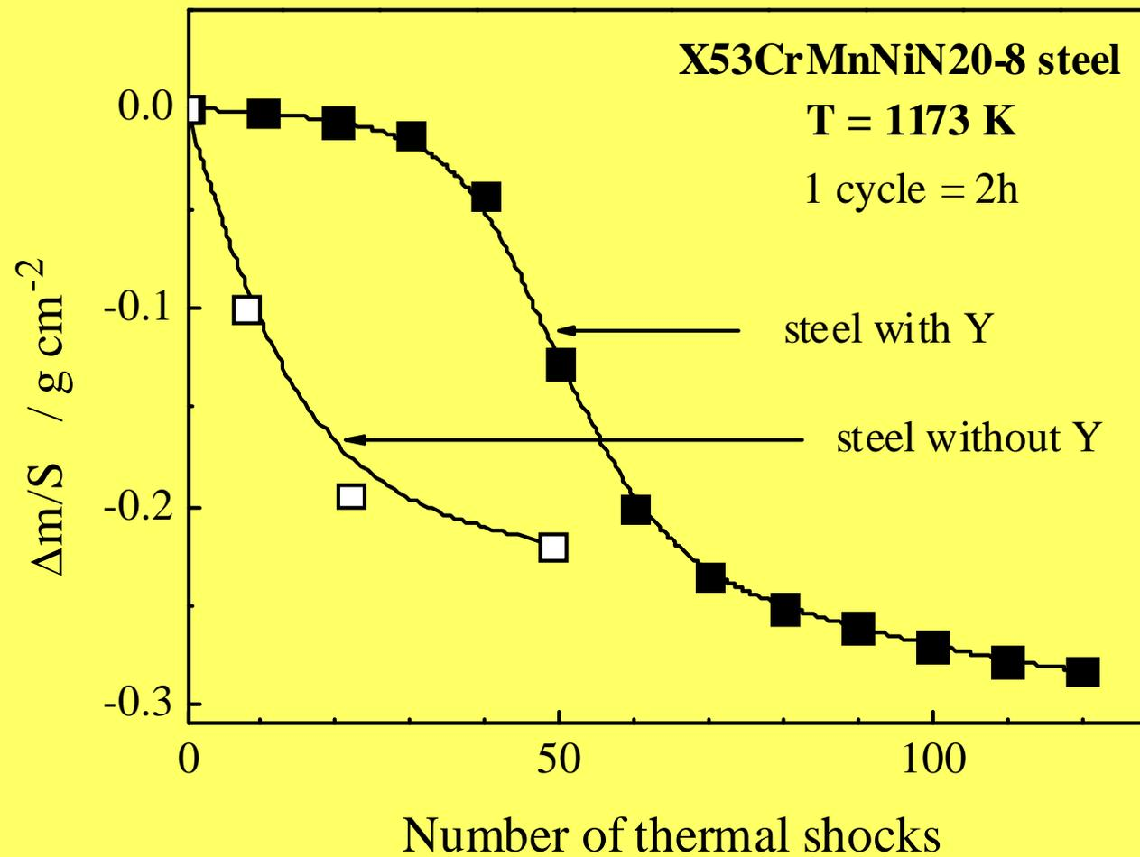
Corrosion behaviour of the X55CrMnNiN20-8 steel uncovered and covered with yttrium under thermal shock conditions
