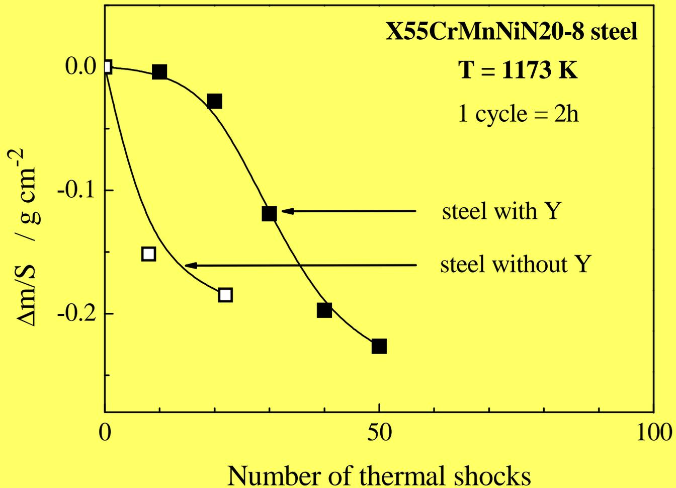
The collective plot, summarizing the results of thermal cycles of four studied steels covered electrochemically with yttrium
