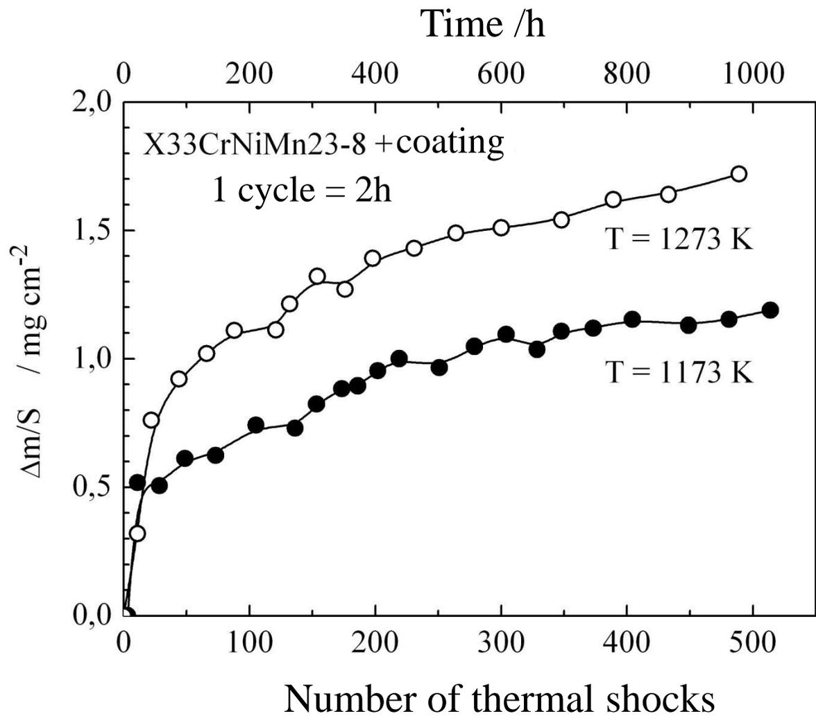
The results of oxidation of two valve steels coated with a protective coating under thermal shock conditions
