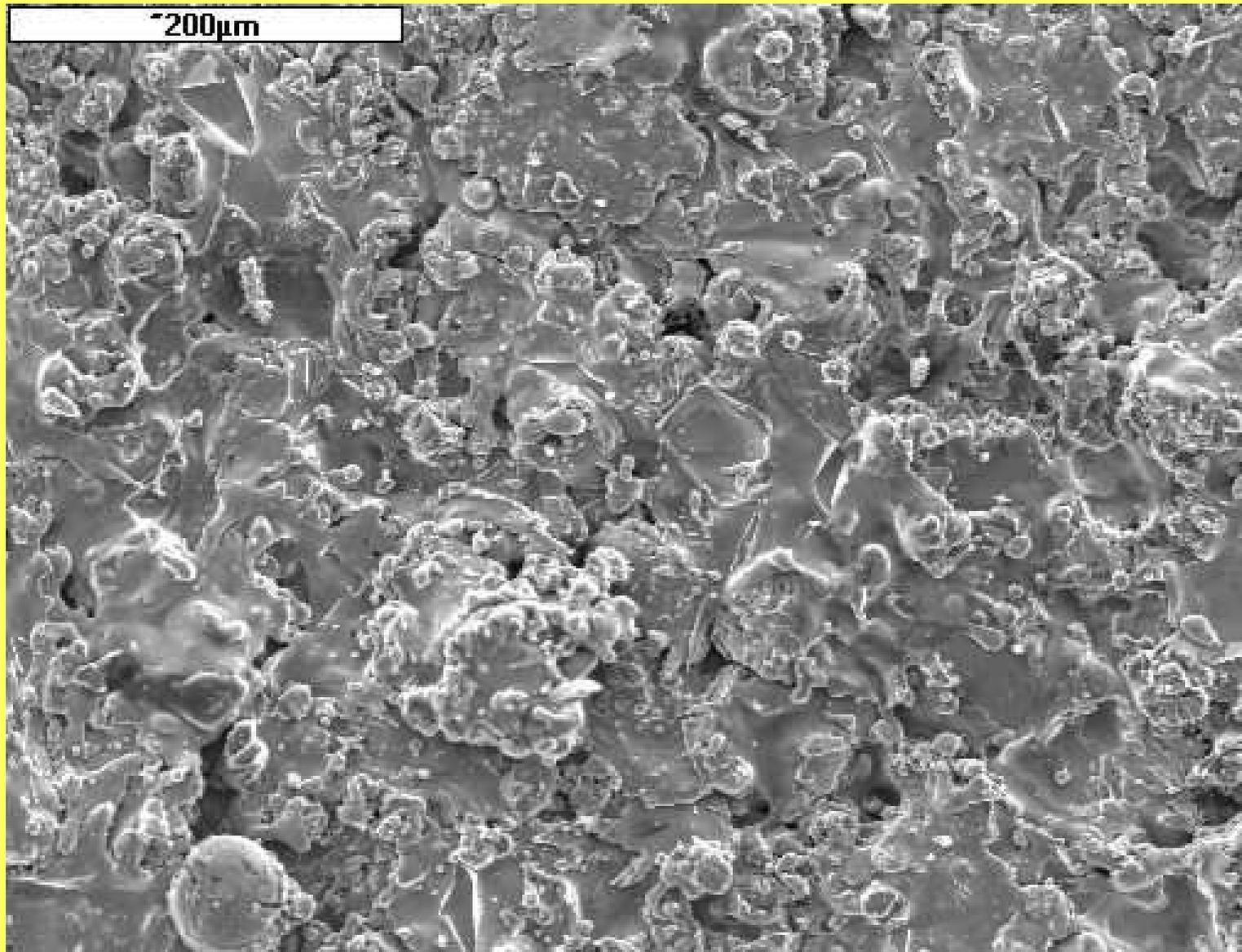
The results of oxidation of X50CrMnNiNbN21-9 steel coated with a protective coating under thermal shock conditions
