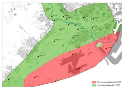
Figure 4. The two areas in which aquifer can be divided due to its improving or worsening of chloride concentration relative to initial concentration.
