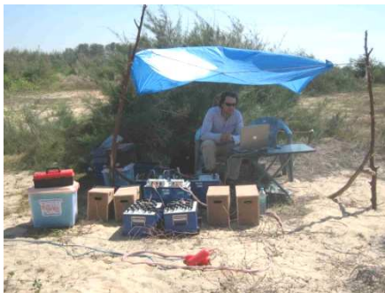
Figure 1. MRS equipment (Numis device from Iris Instrument).
