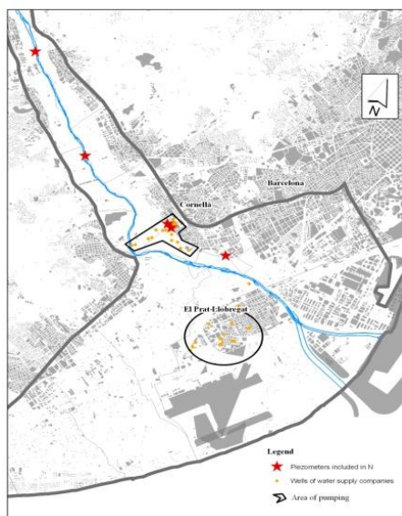
Figure 1. Situation of piezometers included in indicator N, and the water supply companies' pumping areas.
