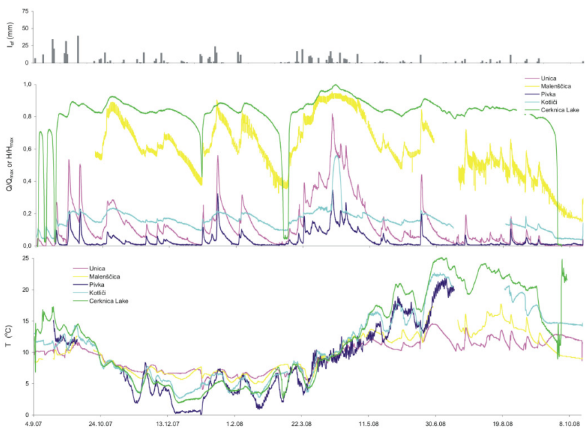
Figure 3. Effective infiltration and discharges or water levels (presented relatively to the maximum value for the two hydrological years) at selected monitoring points in the first hydrological year 2007-2008.
