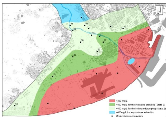
Figure 5. Aquifer can be divided according to the final chloride concentration: blue area in which chloride concentrations are less than 400 mg/L for any volume extraction; red zone in which chloride concentrations are over 400mg/L for any volume extraction; and green zone in which chloride concentrations are less than 400 mg/L when volume extraction is less than the indicate pumping beside the points.
