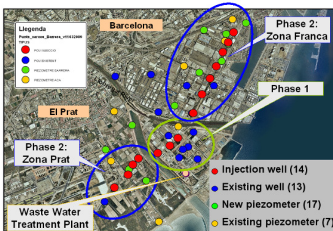
Figure 3. Hydraulic barrier network configuration: injection wells (red) and monitoring points (blue, green and orange). The project has been performed in two phases.
