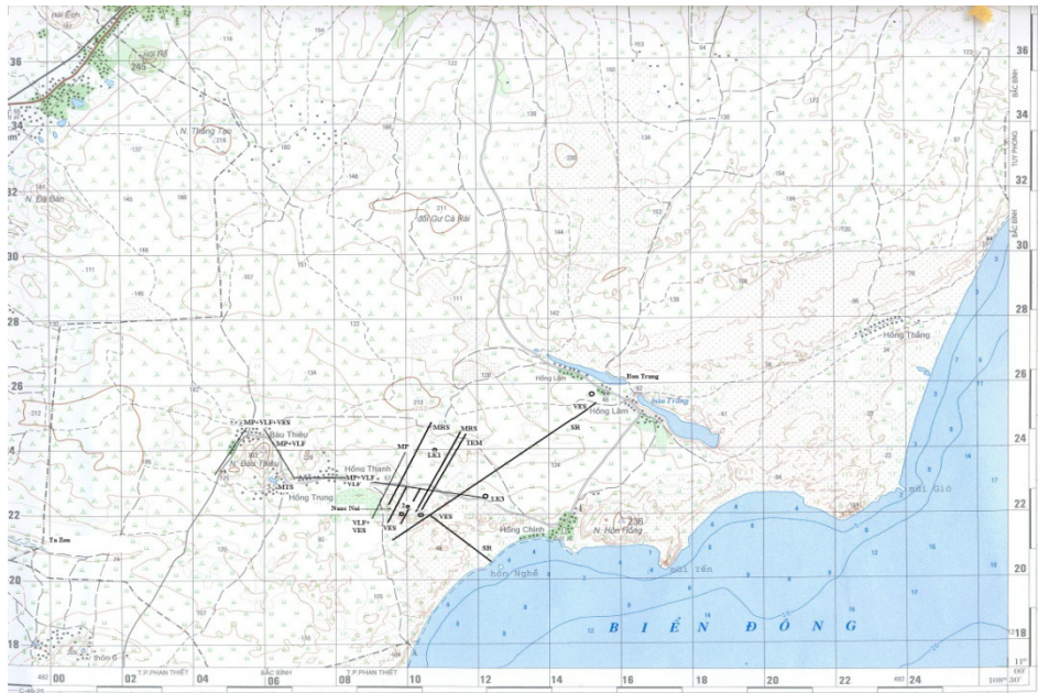
Figure 1. The location of geophysical stations and profiles on the sand dunes studying area Binh Thuan, Vietnam (VES — Vertical Electrical Sounding; EP — Electrical Profiling; VLF — Very Low Frequency; MTS — Magnetotelluric Sounding; MP — Magnetic Prospecting; MRS — Magnetic Resonance Sounding; TEM — Transient Electromagnetic Method; SR — Seismic Refraction; LK1 — Well number 1).
