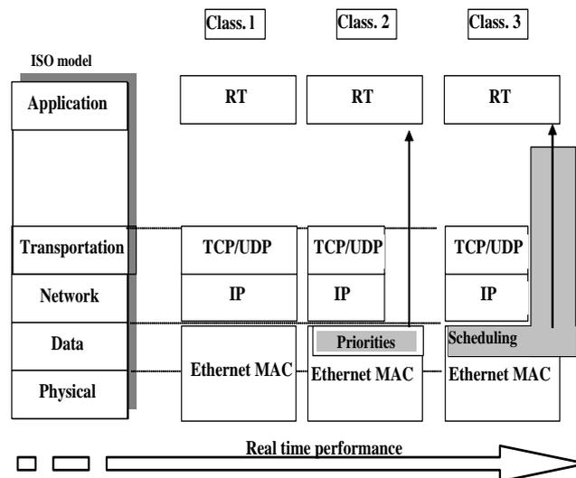
Fig.2.2 Classification of industrial Ethernet (IEC 61 784-2)
