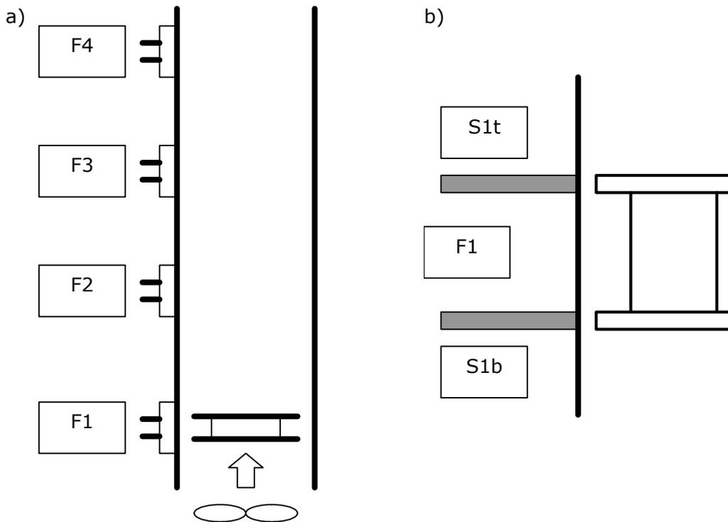
Fig. 5.3. Aero-Lift test rig: a) system overview, b) floor configuration
