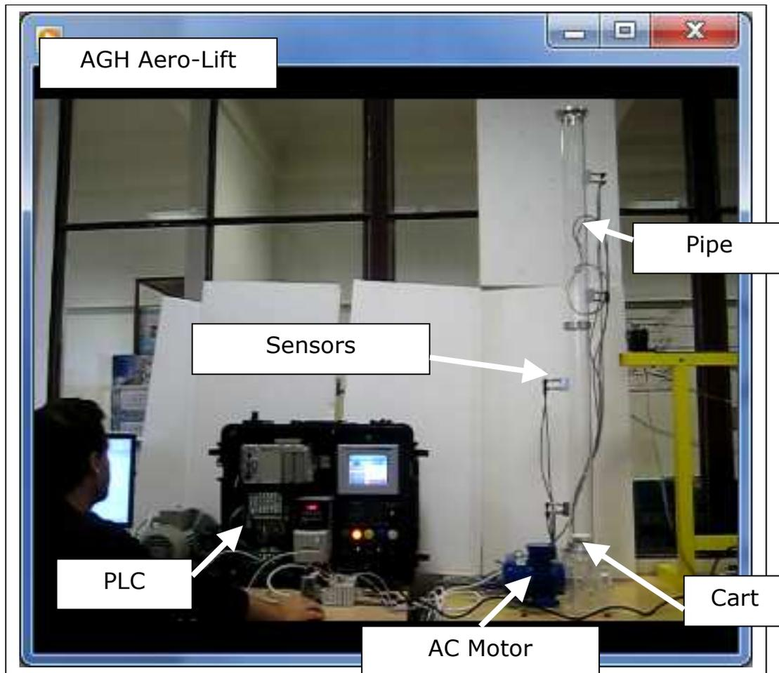
Fig. 5.2. Aero-Lift - laboratory test-rig
