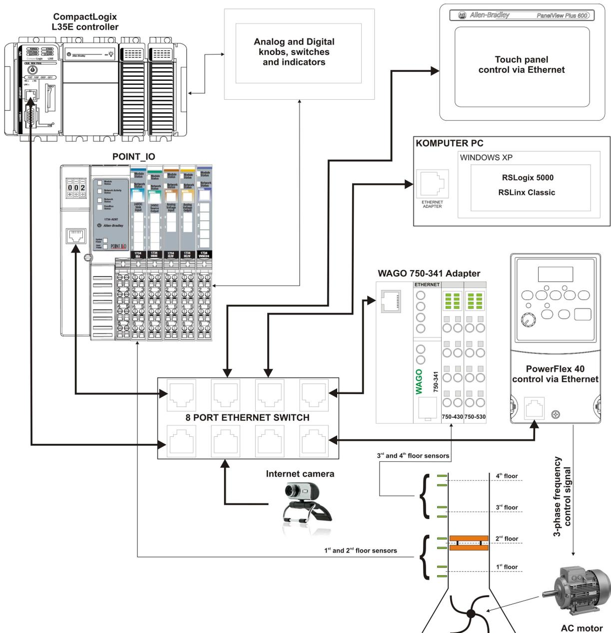
Fig. 5.1. Schematic diagram of the laboratory setup
