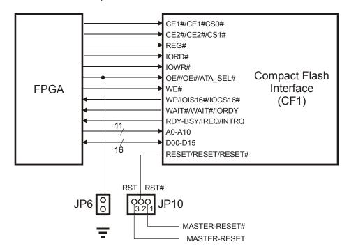
Depending upon the mode in which the Compact Flash card is to be accessed, the shunts on jumpers JP6 and JP10 must be set as follows:
