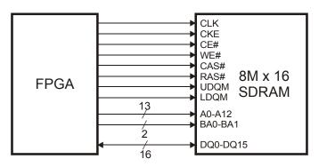
The FPGA has access to an 8M x 16 SDRAM from Hynix (<u>HY57V281620HCT-H</u>) or Samsung (<u>K4S281632E-TC75000</u>) for storing larger amounts of data.
