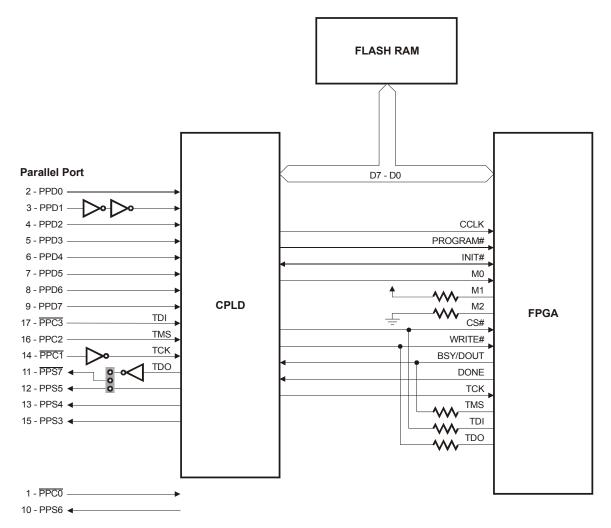
After the FPGA is configured with a bitstream and the DONE pin goes high, the CPLD switches into a mode that connects the parallel port data and status pins to the FPGA. For more details on how the CPLD manages the interface between the parallel port and the FPGA both before and after device configuration, see the XSB Parallel Port Interface application note.
