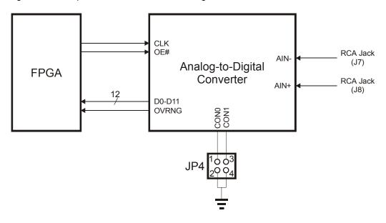
The ADC supports several operating modes determined by the arrangement of the shunts on jumper JP4:
