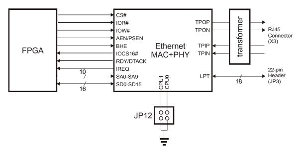
The Ethernet chip supports several microprocessor bus interfaces. The interface is chosen by setting the shunts on jumper JP12 as follows:
