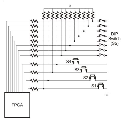
The table below lists the connections from the FPGA to the switches. The DIP switches also share the same pins as the uppermost eight bits of the Flash RAM address bus. If the Flash RAM is programmed with several FPGA bitstreams, then the DIP switch can be used to select a particular bitstreams which will be loaded into the FPGA by the CPLD on power-up.
