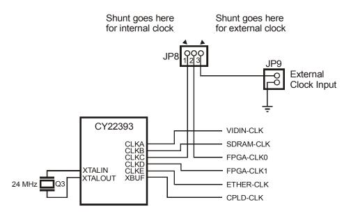
To sync the XSB circuitry with an external system, you can insert an external clock signal through jumper JP9 and place a shunt at position "EXT" of jumper JP8. This external clock replaces the FPGA-CLK0 output from the oscillator.
