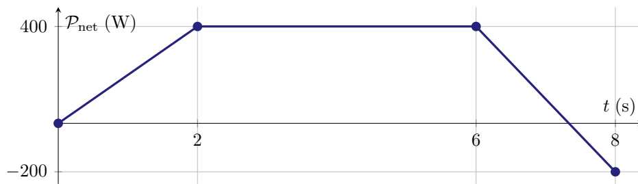
Figure 7.36: Problem 36: a signed net-power history. Every connecting segment is straight; the area under the graph is net work. Kinetic energy reaches its maximum when the final descending segment crosses zero power.
