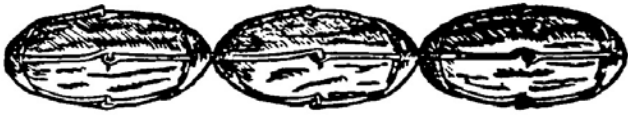
Figure 4 — Gilbert's method of 'arming' lodestones to improve their attractive force by attaching soft iron caps
