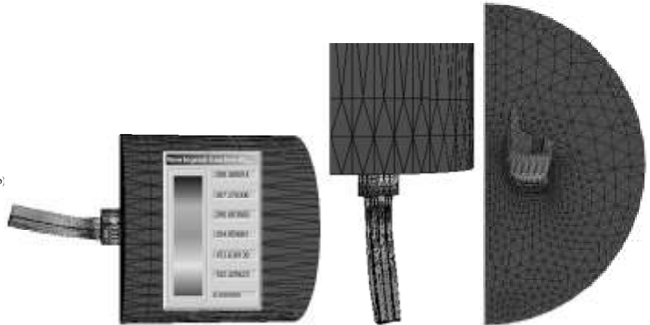
Bend of the profile and longitudinal velocity component distribution in deformation zone during extrusion with out working bend.
