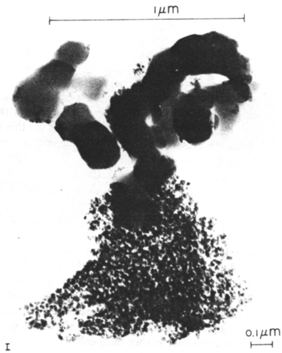
Electron micrograph of alumina I agglomerates.
