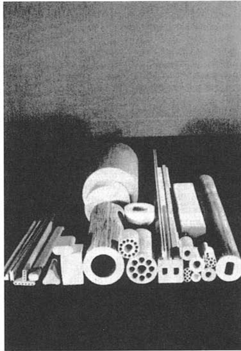
FIGURE 13.52 A variety of ceramic parts that have been fabricated by extrusion. (Photo courtesy of Superior Technical Ceramics Corporation, St. Albans, VT.)
