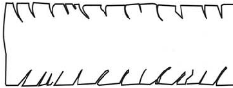
FIGURE 13.54 Drawings of the cross section of an extruded part illustrating the appearance of tearing. (From Robinson, G.C., Extrusion defects , in Ceramic Processing Before Firing , Onoda, G.Y. and Hench, L.L., Eds., Wiley-Interscience, New York, 1978. With permission.)
