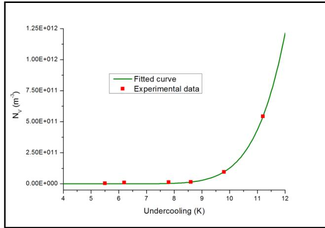
Fig. 7.  $N_V$  on undercooling dependence for 76  $\mu\text{m}$  particles.
