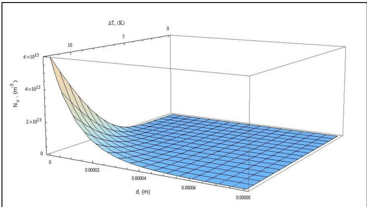
Fig. 8.  $N_V$  dependence on undercooling and mean grain diameter.
