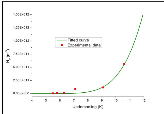
Fig. 6.  $N_V$  on undercooling dependence for 40  $\mu\text{m}$  particles.
