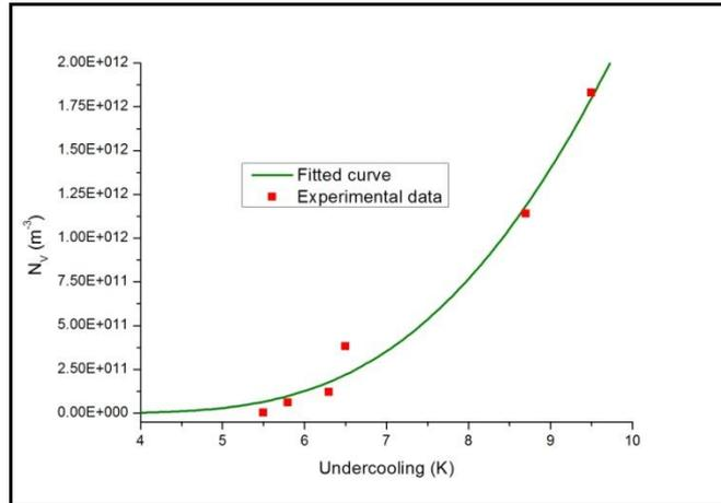
Fig. 5.  $N_V$  on undercooling dependence for 10  $\mu\text{m}$  particles.
