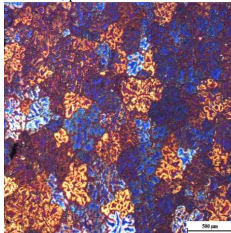
Fig. 2. 2% of SiC, particles mean diameter 40  $\mu\text{m}$ ;
