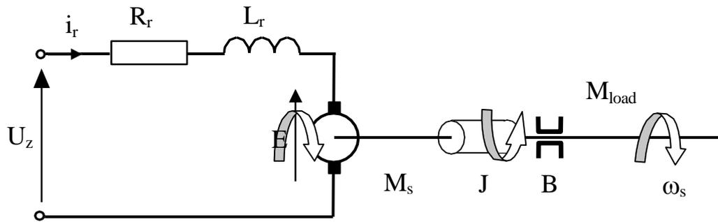
Fig. 2.2 DC Motor Rotor Circuit Equivalent Diagram
