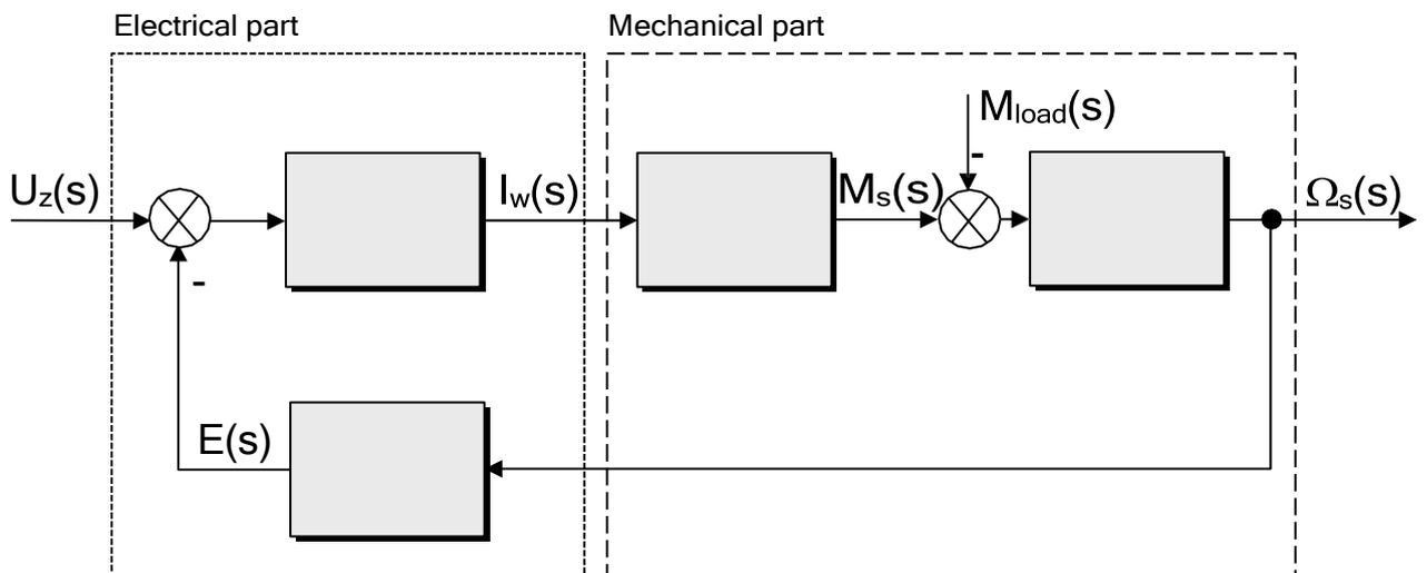
*Fig. 2.3 DC motor block diagram*
