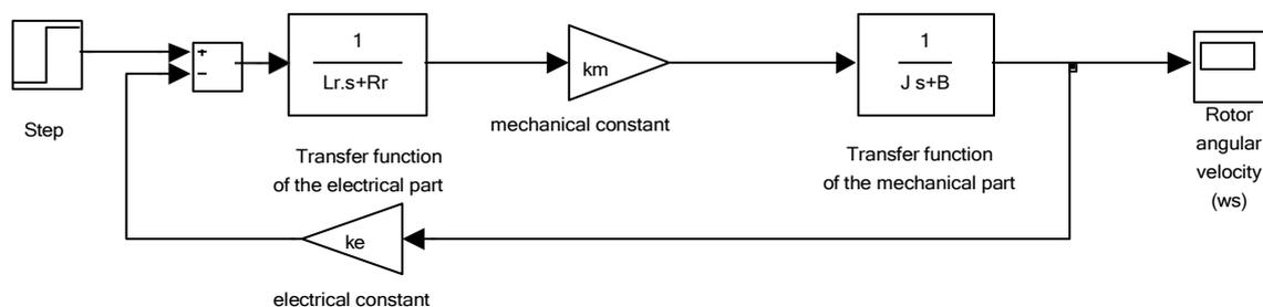
Fig. 2.5 Motor block diagram built in Simulink
