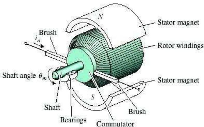
Fig. 2.1 Construction of a permanent magnet DC motor
