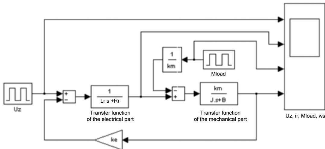
Fig. 2.7 Motor block diagram built in Simulink
