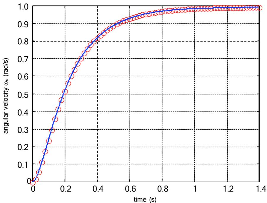
Fig. 2.6 Step response of a DC motor, obtained using:
