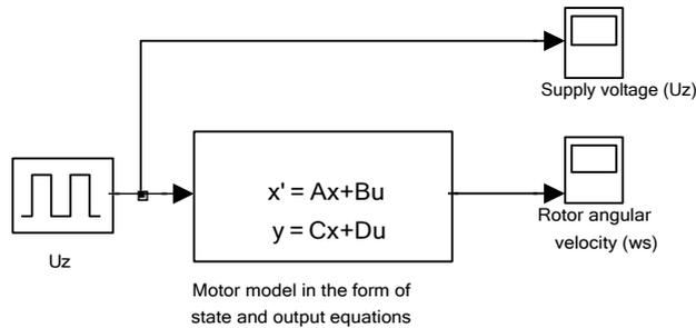
Fig. 2.9. Motor block diagram built in Simulink
