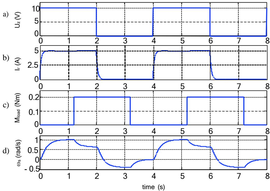
Fig. 2.8. Waveforms obtained during simulation: a) rotor supply voltage ( $U_z$ ), b) rotor current ( $i_r$ ), c) motor load torque ( $M_{load}$ ), d) rotor angular velocity ( $\omega_s$ )
