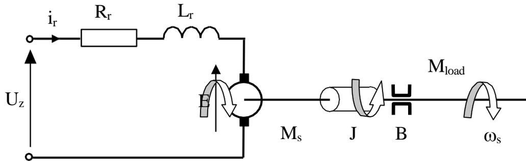
Fig. 2.2 DC Motor Rotor Circuit Equivalent Diagram
