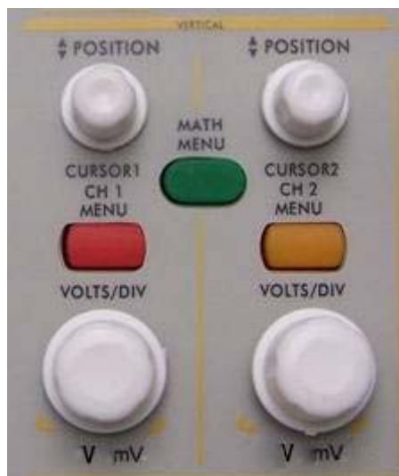
Fig. 4-9 Vertical Control Zone
