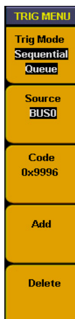
Fig.5-60: Sequential queue trigger
