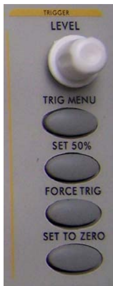
Fig.4-11 Trigger Control Zone
