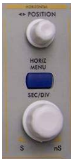
Fig. 4-10 Horizontal Control Zone
