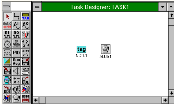
Figure 3-34 Add alarm block and TAG block
