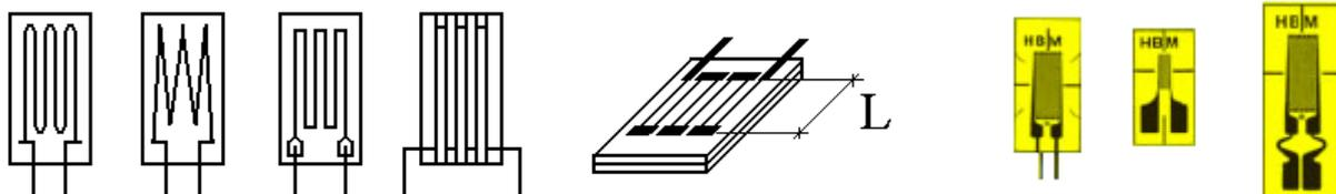
Grid shaped strain gauges are insensitive on transverse deformation which is its advantage over loop shaped gauges. Each sensor ends with a copper ending of much larger cross-section and very low resistance – they allow connecting (i.e. soldering) the sensors with proper gauges. Few types of endings proposed by HBM company are visible above.
