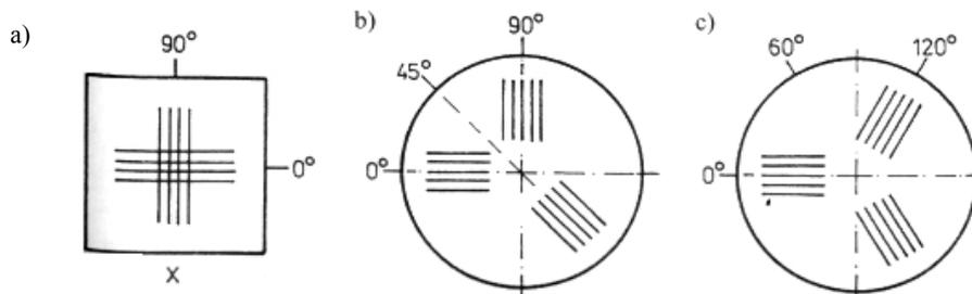
a) two-gauge rosette    b) perpendicular rosette ( $0^\circ/45^\circ/90^\circ$ )    c) delta type rosette ( $0^\circ/60^\circ/120^\circ$ )
