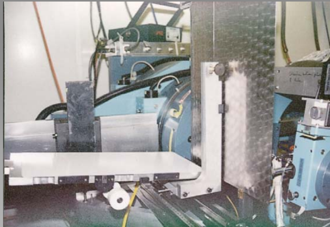
Rear view of TIP camera mounted at X7B, NSLS, BNL
