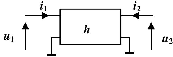
$$\begin{cases} u_1 = h_{11}i_1 + h_{12}u_2 \\ i_2 = h_{21}i_1 + h_{22}u_2 \end{cases}$$
