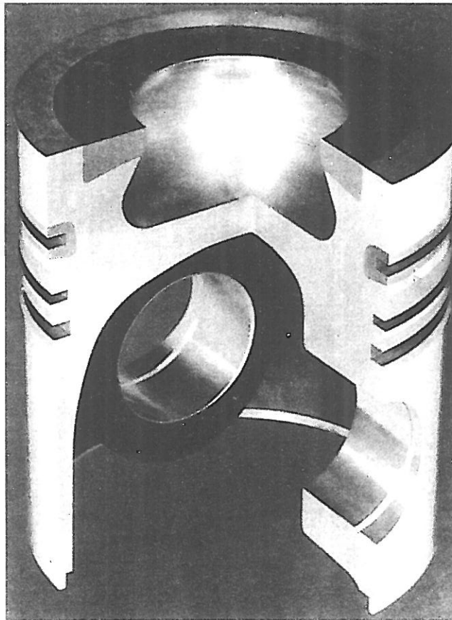
Fig. 1. A Diesel engine piston, squeeze cast, with the reinforced crown part enclosing the combustion chamber. The ceramic preform based on short alumina fibers was used (TOYOTA-Japan)
