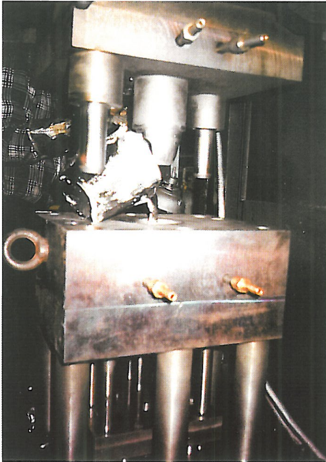
Fig. 47. Pouring of the die cavity with liquid particulates reinforced composite. The four ends visible on the photograph are used for connecting the water or air feeding pipes to the cooling system.
