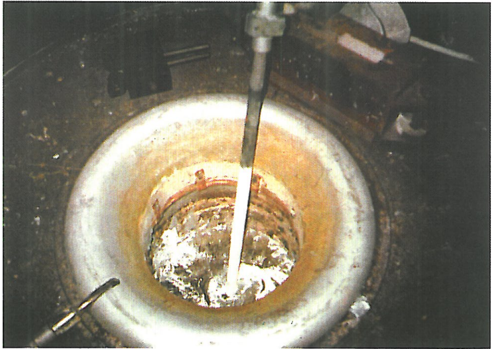
Fig. 40. Mixing of the liquid particulates reinforced composite to obtain a homogeneous distribution of reinforcing phase in the metal matrix
