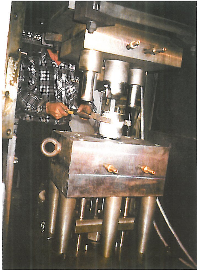
Fig. 50. The ejection of a ready squeeze composite casting from the die
