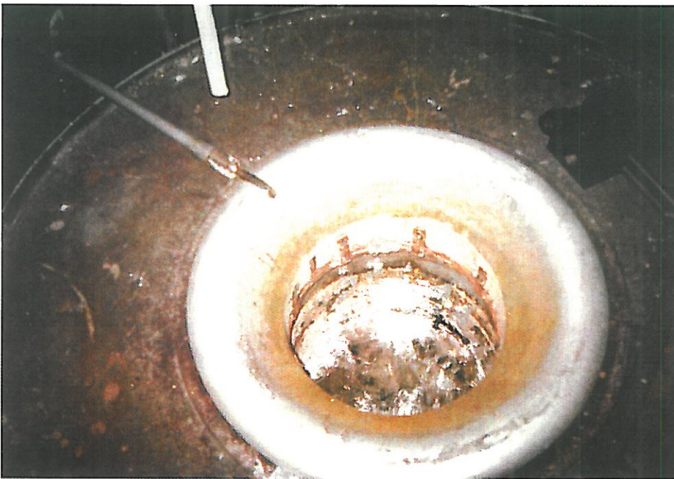
Fig. 41. A crucible with the liquid particulates reinforced composite. The operation of mixing completed. The liquid composite is ready for further recycling
