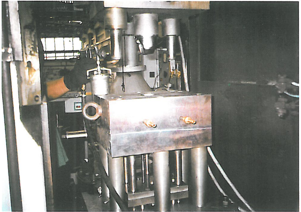
Fig. 46. Application of protective and parting coatings on the working surfaces of a die for squeeze casting of composite pistons
