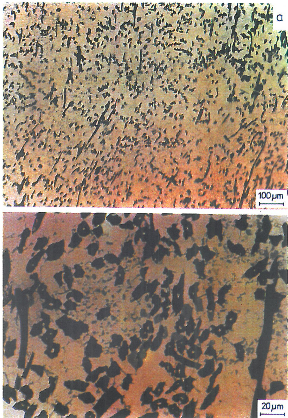
Fig. 57. Microstructure of aluminium alloy – Polish carbon felt composite obtained by squeeze casting in the Foundry Research Institute (a), structure of fibre preform (graphite felt) (b), and fracture of AlSi12CuMgNi+ graphite felt composite (c) made by squeeze casting in the Foundry Research Institute, Kraków
