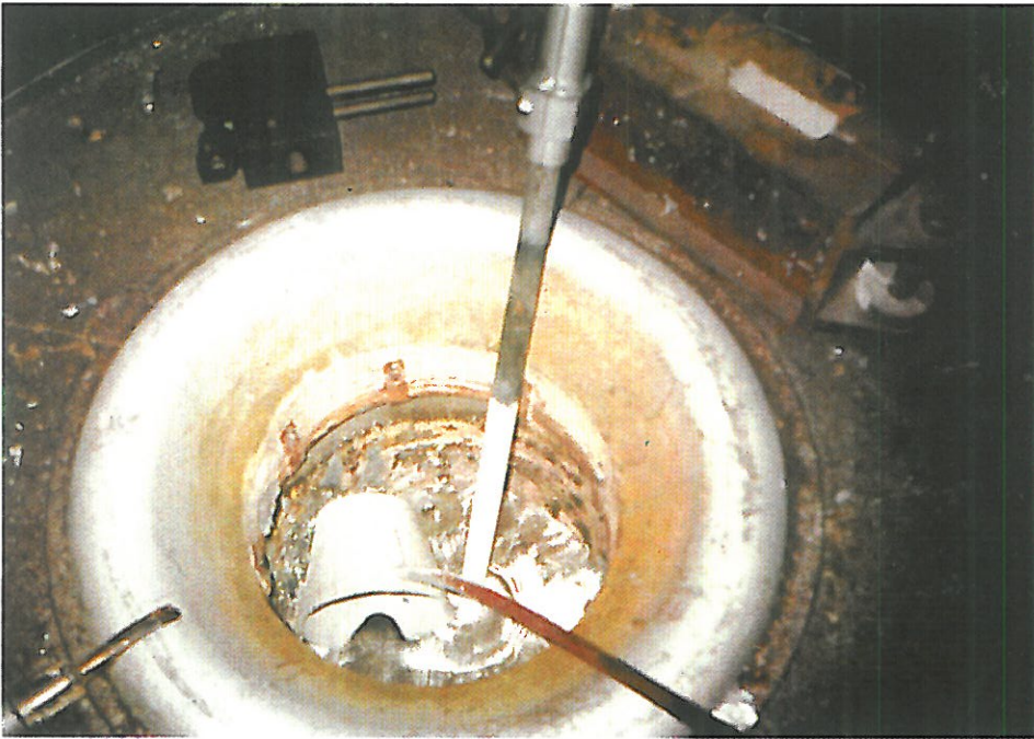
Fig. 43. When casting composites with a reinforcing phase susceptible to settlement or flotation it is possible to scoop up a portion of the liquid composite for further recycling even during the operation of mixing under the cover on inert gas
