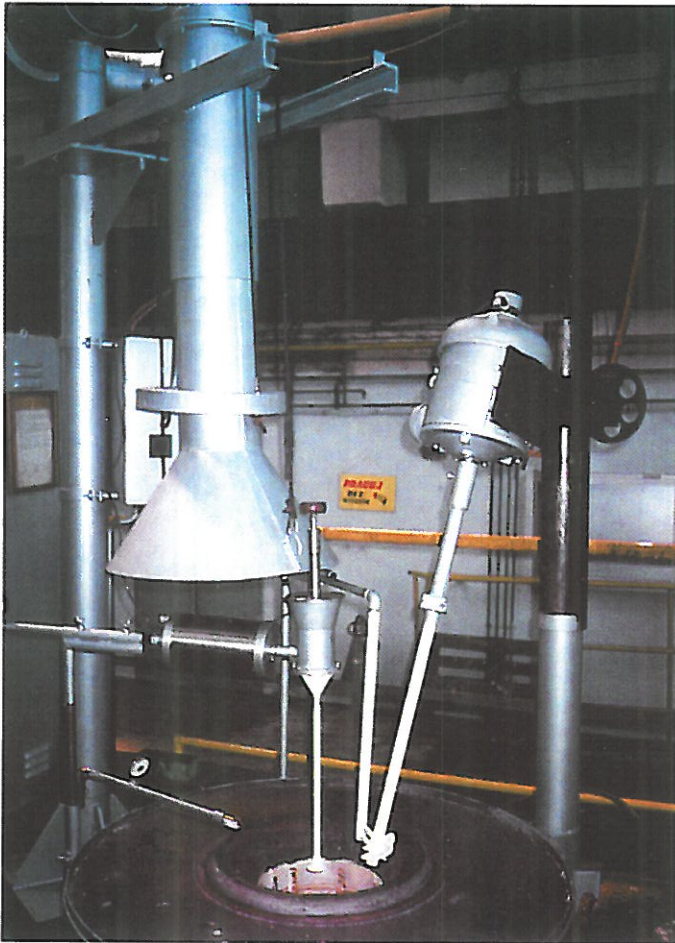
Fig. 37. The stand for fabrication of cast metal matrix composites in the Foundry Research Institute, Krakow. The stand comprises an installation for homogenization of metal liquid under the cover of argon (on the left) and a 160 t capacity hydraulic press for squeeze casting, equipped with a die, a device for spray application of protective and parting coatings, and a set of measuring instruments for control of the thermal and force-related process parameters
